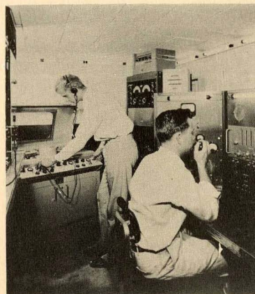
Illust. 16. Ruggedized recorder in a mobile application (part of telemetry van).
