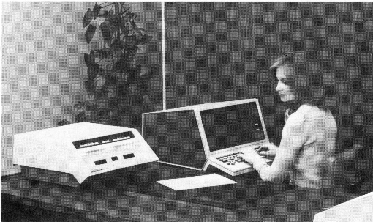
Figure 2. Tape Cassette System With UNISCOPE 200 Display Terminal
