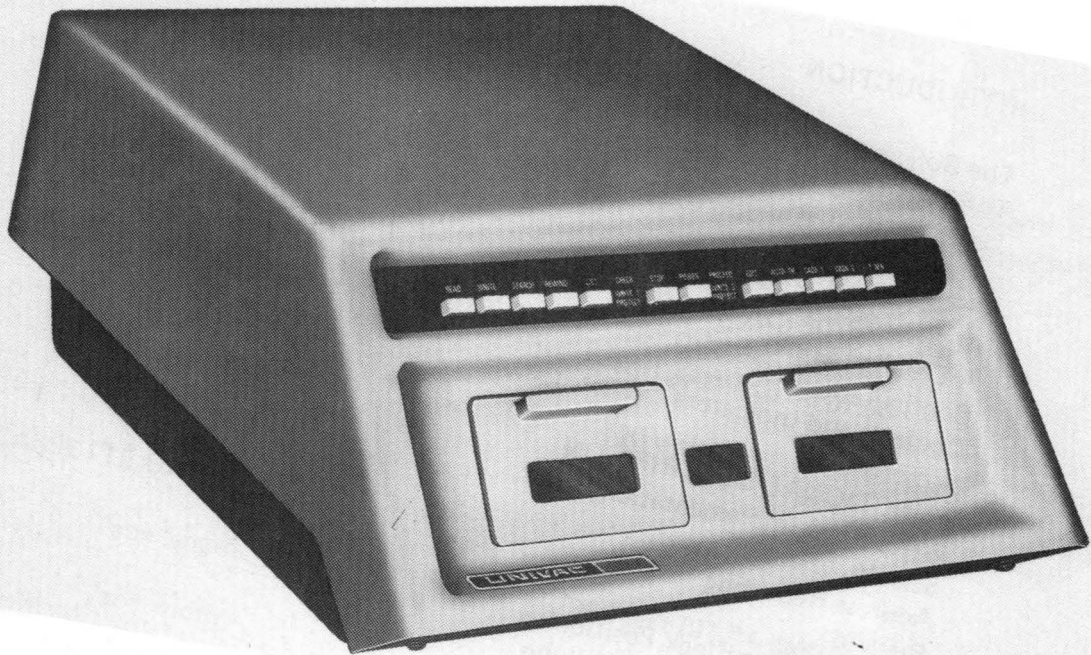
Figure 1. SPERRY UNIVAC Series 600 Tape Cassette System
