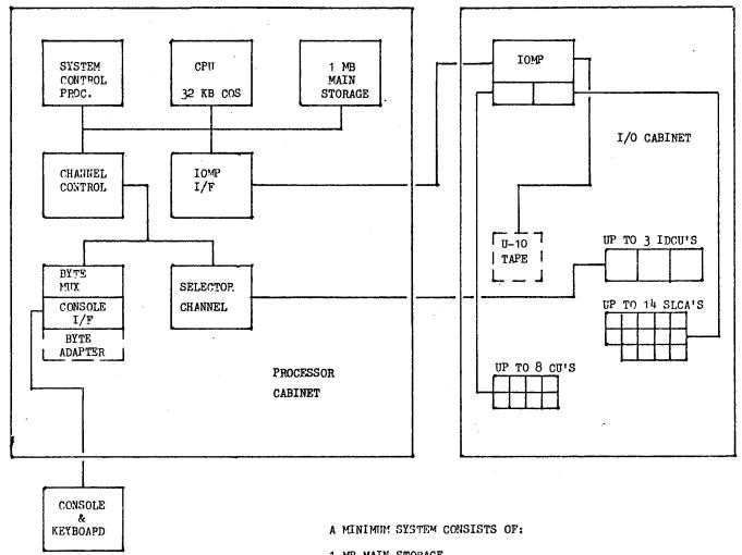
NOTE: -IDCU - Integrated Disk Control Unit for 8416/ 17,18,19 8470 Disks - SLCA - Single Line Communication Adapter - IOMP - Input-Output
