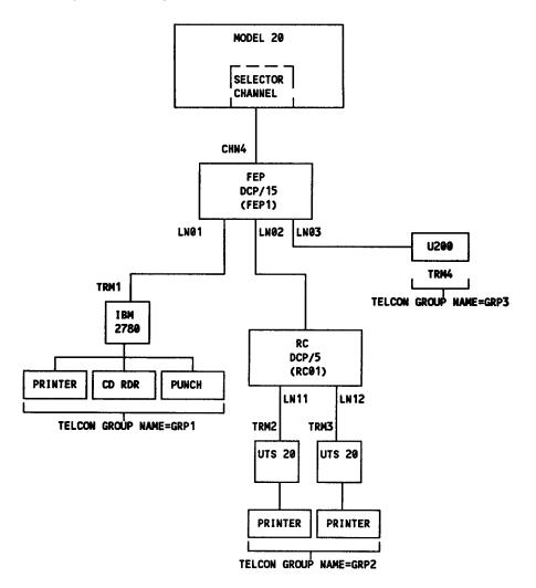
This network could be defined as indicated below. Line numbers are provided to correlate the network definition with the explanation that follows:
