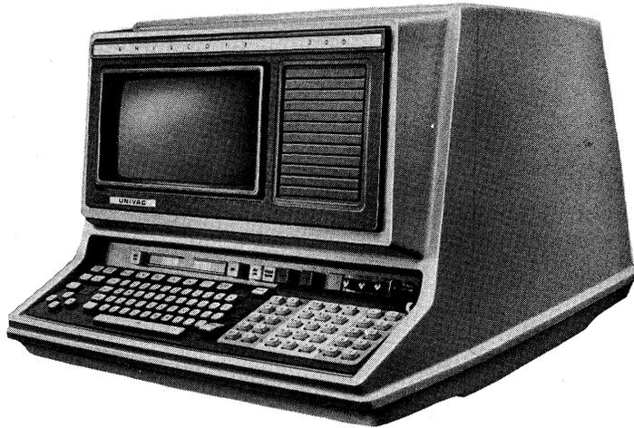
The UNIVAC UNISCOPE 300 Visual Communication Terminal Subsystem is designed for applications requiring direct user interaction with the central system. These terminals can be located at or near the site, or they may be operated as remote stations over standard data communication facilities.
