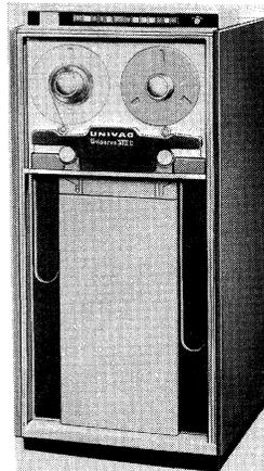
A UNISERVO VIII-C Subsystem can have up to 16 magnetic tape units, and can incorporate either one or two control units attached to one or two input/output channels for single or dual channel operator.
