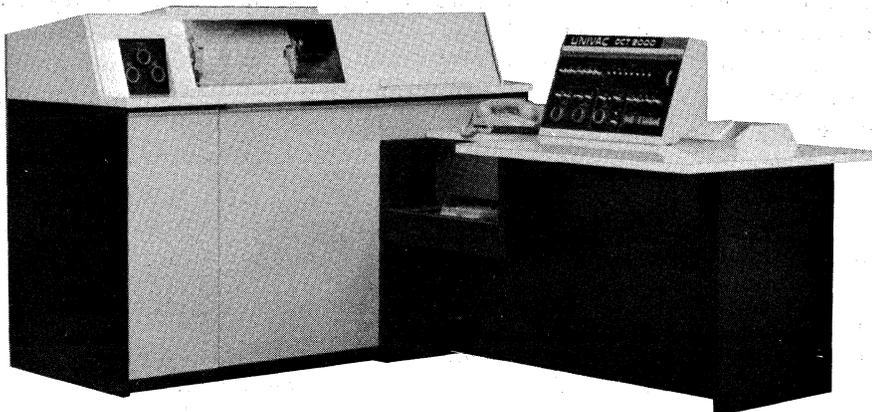
The UNIVAC Data Communication Terminal (DCT) 2000 is a combination printer and card reader/punch designed to transfer large quantities of data efficiently over voice-grade facilities. This terminal, tied into a network with computers (the UNIVAC 1004 Card Processors or other DCT 2000 systems), can handle up to 250 blocks per minute. The DCT 2000 is also available without the combination card reader/punch for use as a printer terminal.
