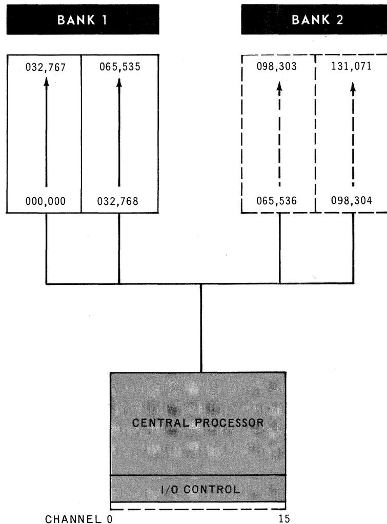
Figure 2-5. Unit Processor System with Noninterleaved Storage
