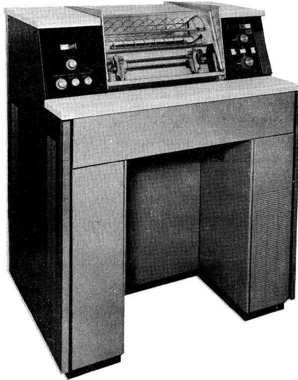
The UNIVAC High Speed Printer Subsystem provides the UNIVAC 1108 System with an output printing unit that is capable of printing single or multiple copies of data. Each line of output data may contain up to 132 printed characters. Printing operations occur on a request acknowledge basis allowing the processor to perform other processing functions while the printer is printing data.
