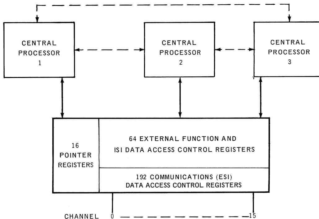
Figure 2-1. The Input/Output Controller
