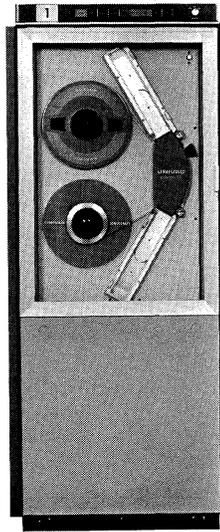
The UNISERVO VI-C Magnetic Tape Unit is a low cost unit having moderate speed and transfer rates for applications involving massive file passing, extensive sorting, or other applications for which high speed magnetic tape subsystems would be desirable.
