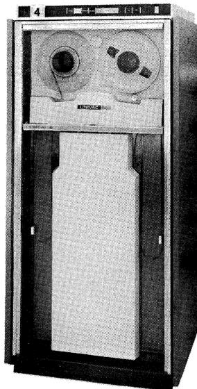
The UNISERVO 16 Magnetic Tape Subsystem is similar to the UNISERVO 12 Magnetic Tape Subsystem except that it has higher performance capabilities. The peak transfer rate is 192,000 frames per second in the primary tape format (9-track, 1600 frames per inch, phase encoding) and 96,000 frames per second in the NRZ format.
