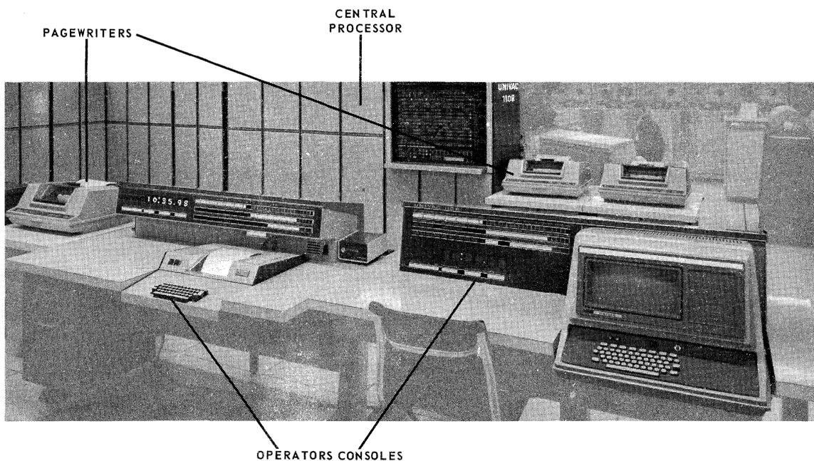
Figure 1-1. The Central Processor and Operator's Console
