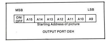
Computer output port OF4 is used to set the format of the TV picture. The function of each of the eight bits of this output port is shown in this table:
