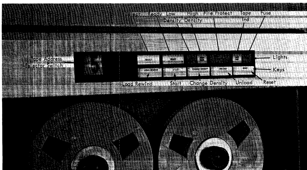
Figure 25. Operating Keys and Lights, IBM 729II and IV
