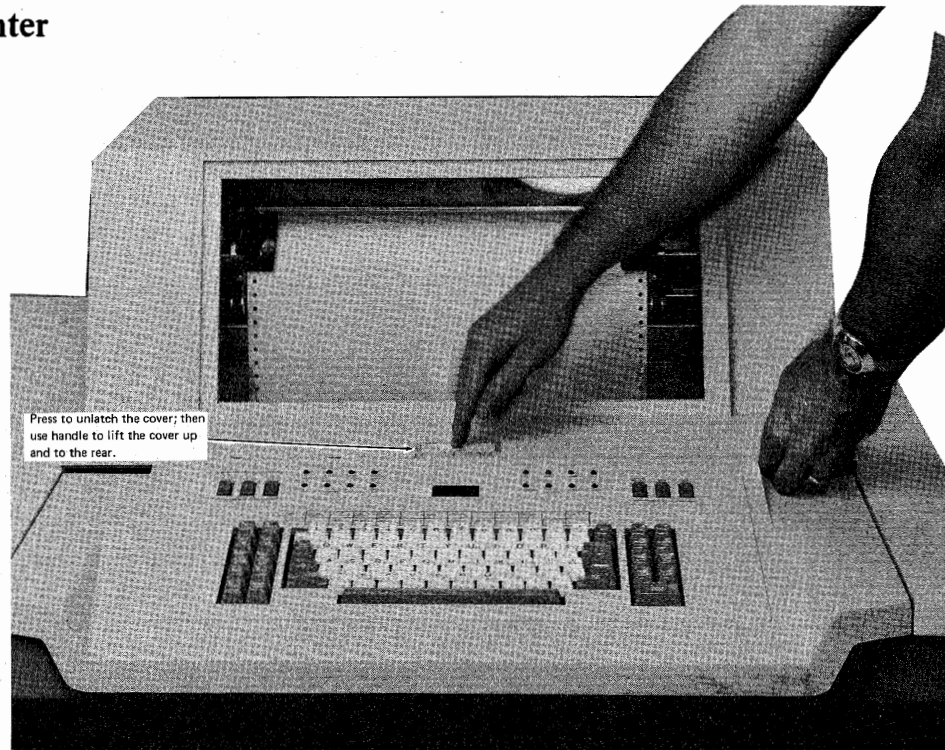
Figure 5-2. Opening the Printer Cover (Part 1 of 2)
