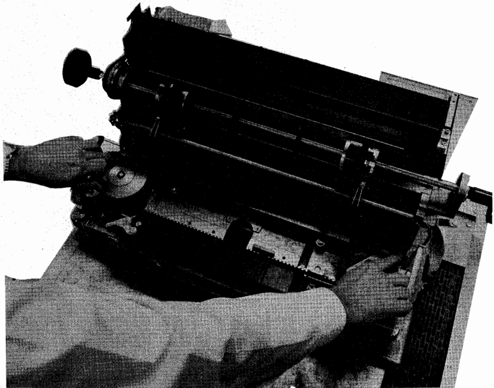
Figure 5-12. Installing the Print Belt
