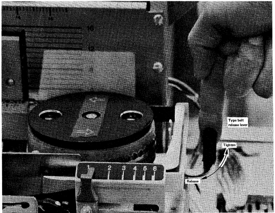
Figure 5-10. Releasing Print Belt Tension
