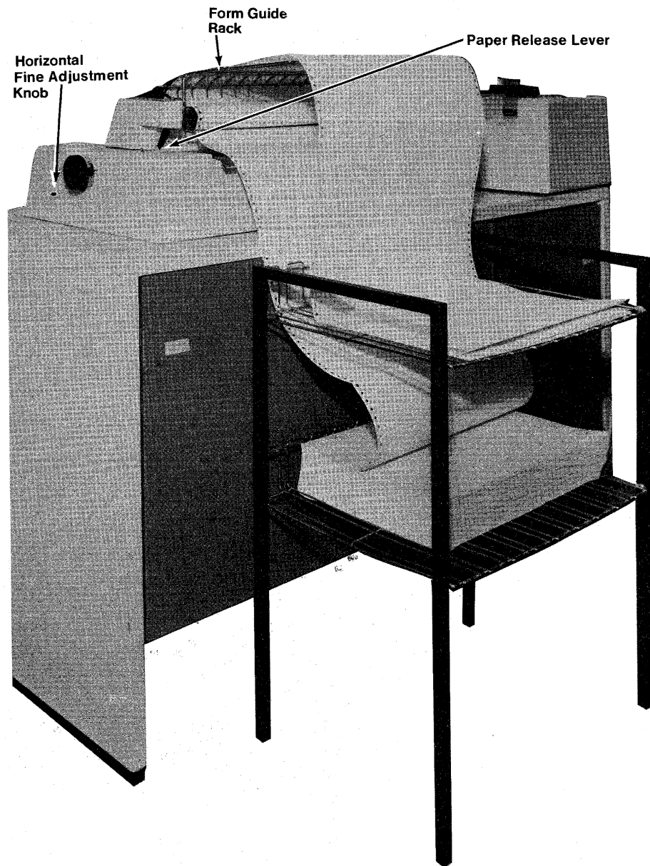
Figure 4-6. Installing Margin-Punched Forms (Part 1 of 2)
