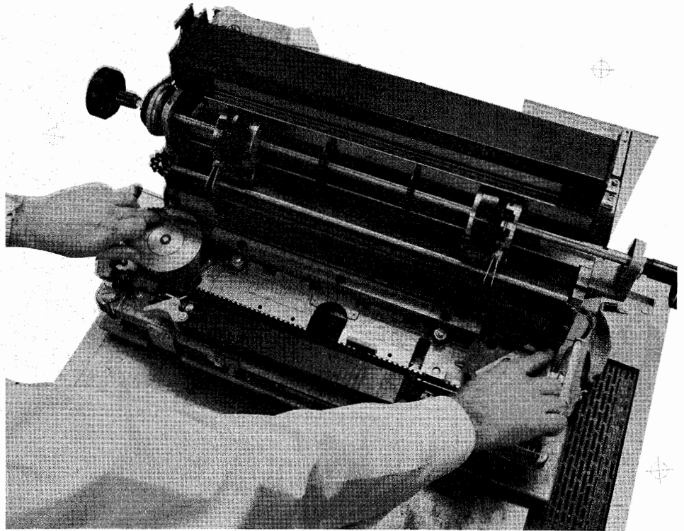
Figure 11-12. Installing the Print Belt
