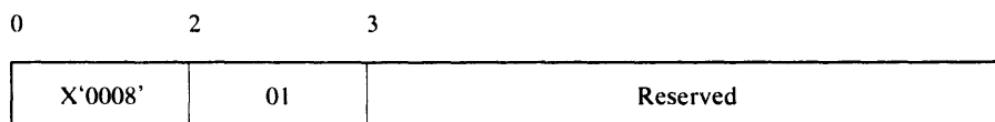
Figure A-7. Special Record at Beginning of Data Records from the Data Component
