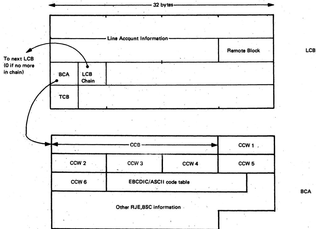
Figure 5.31. RJE Line Control Block and Buffer Control area
