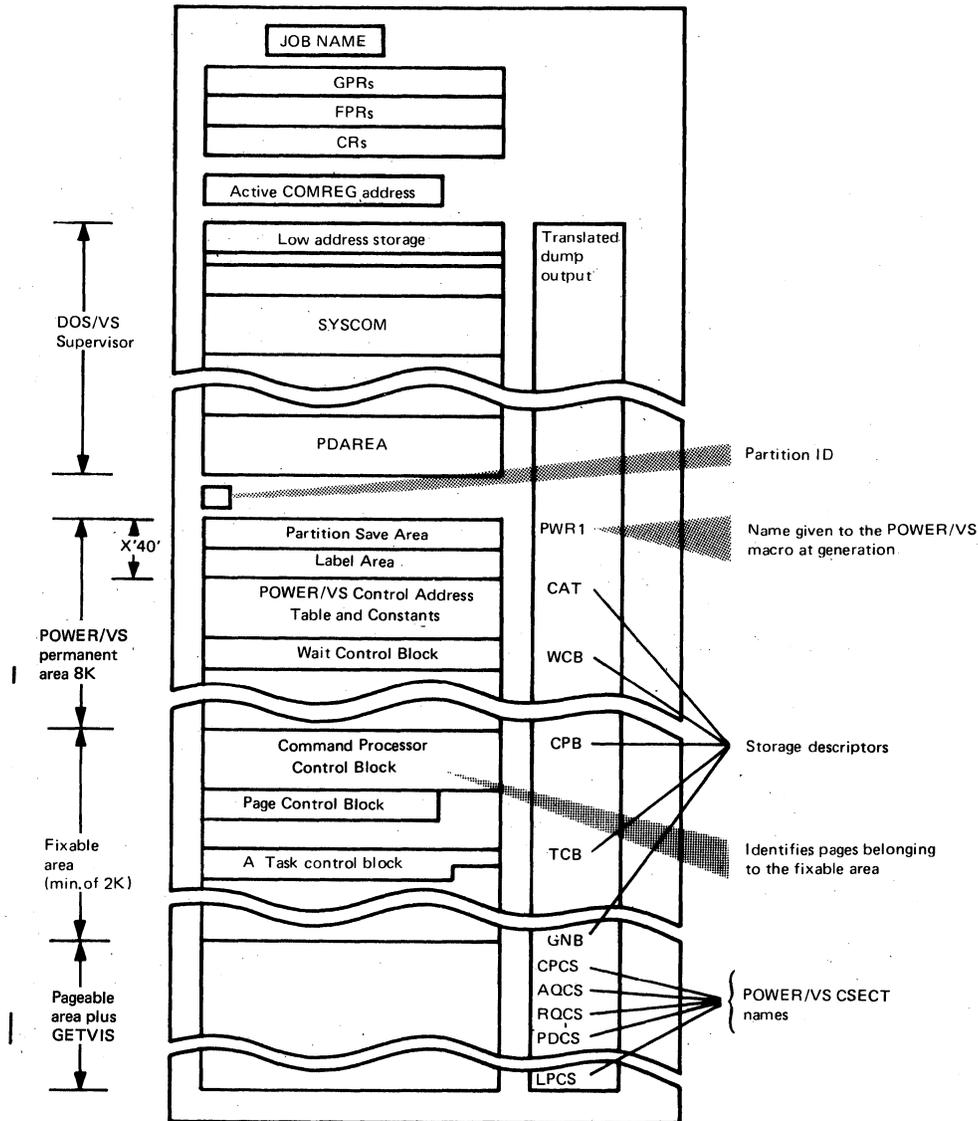
Figure 6.2. Pictorial representation of a system dump containing the POWER/VS partition
