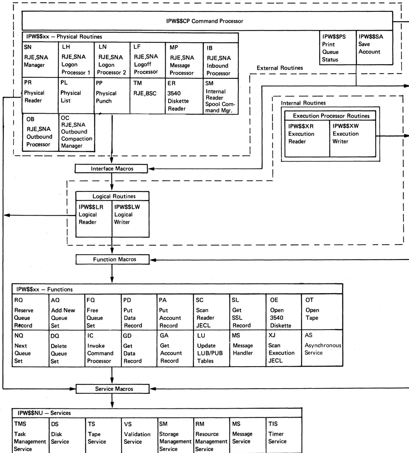
Figure 2.1. Hierarchic organization of calling sequence and interfaces between the POWER/VS routines
