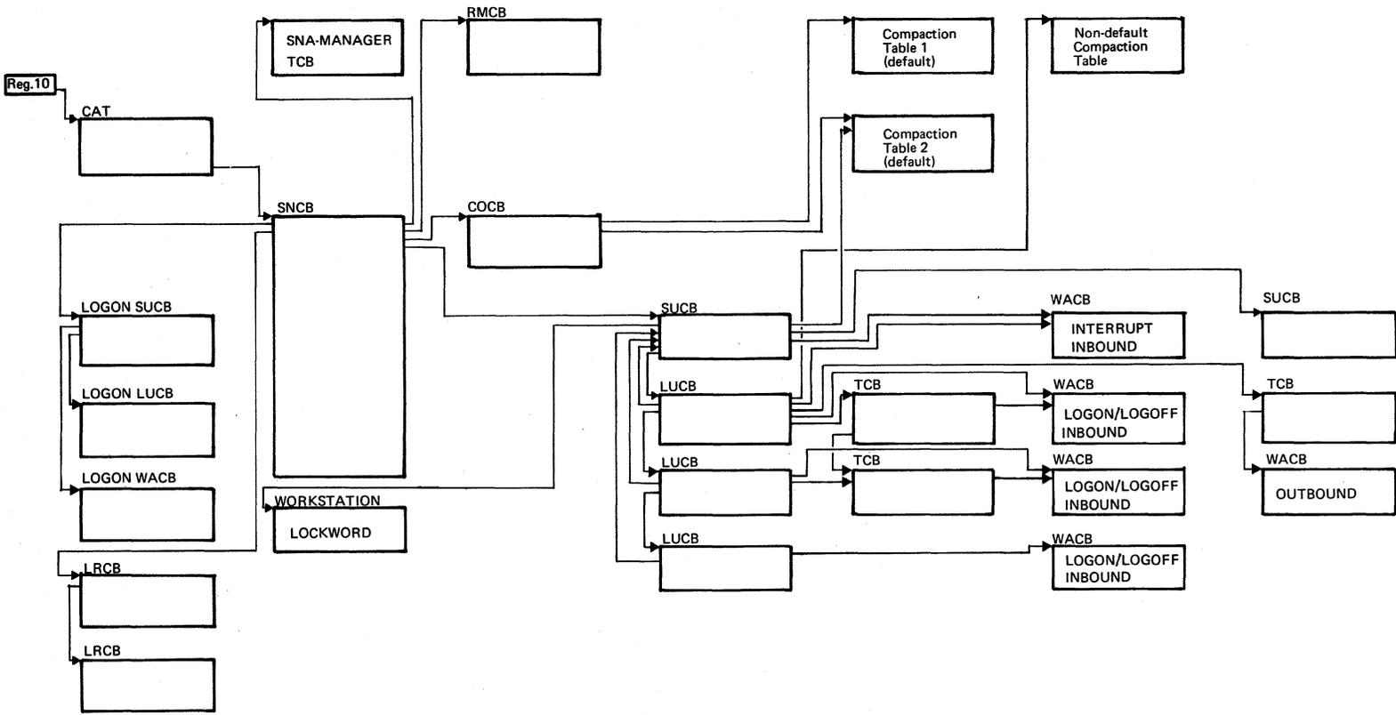
Figure 2.24H. RJE, SNA Control Block and Work Area Chaining
