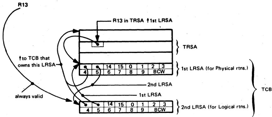
Figure 5.14. Part 1: Linkage between the two LRSAs in a Double Linkage Register Save Area (case 1)
