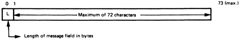
The message field may contain variables for which the message modification routine in the message module (IPW\$\$MS) will substitute the appropriate fields.
