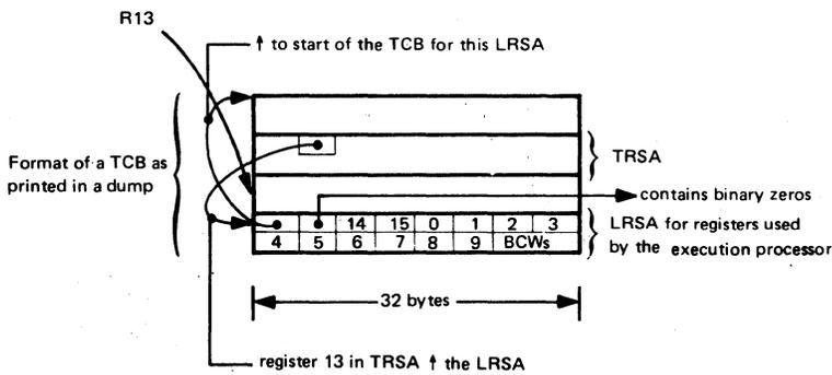
Figure 5.14. Part 3: Linkage from an Execution Processor XR/XW routine
