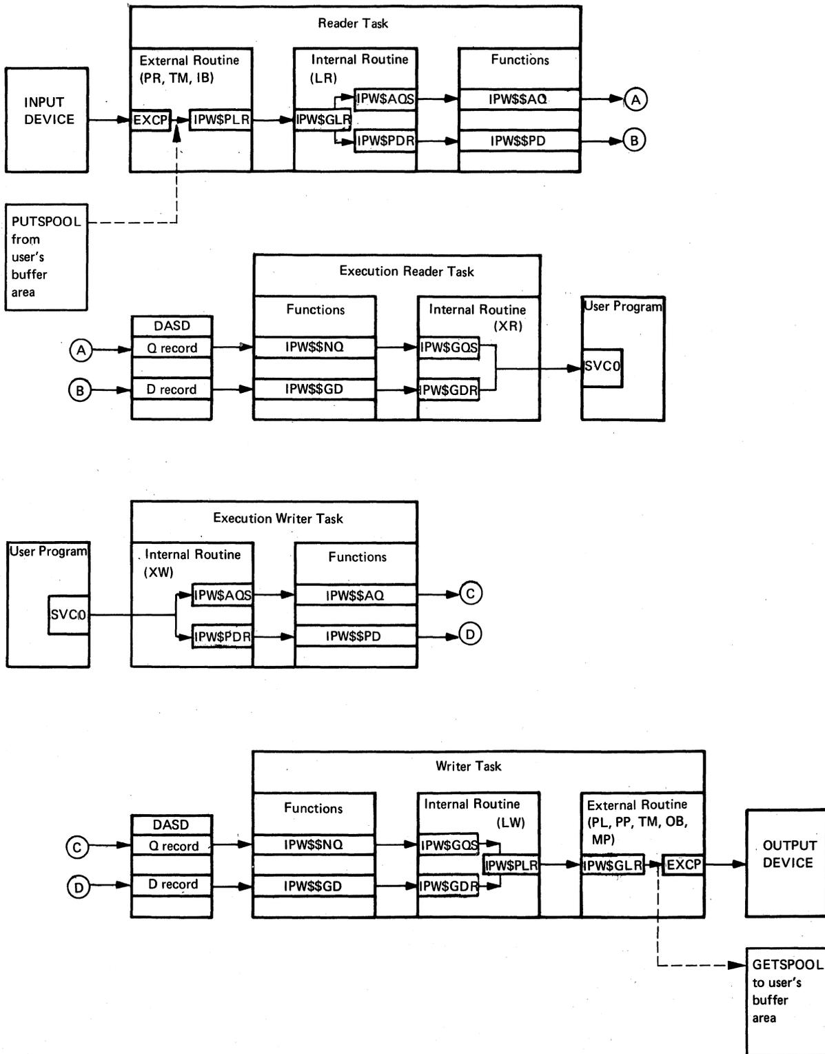
Figure 2.8. Data flow throughout the spooling process
