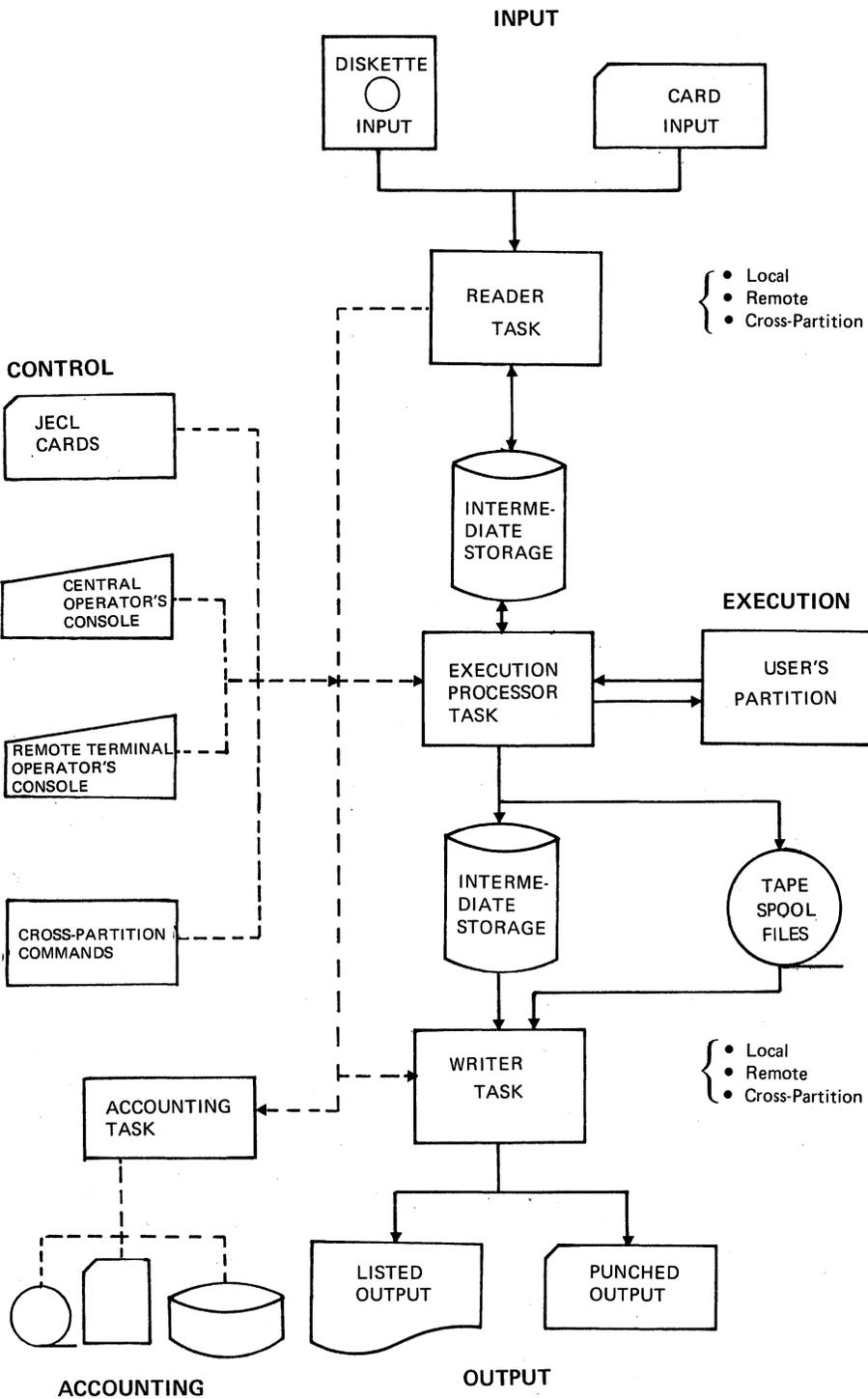
Figure 1.1. The major functions of POWER/VS, data flow, and operator communication
