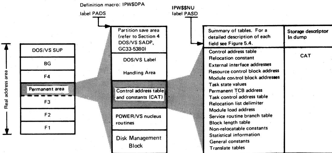
Figure 5.1. Organization of the POWER/VS Permanent Area and the Control Address Table (CAT)
