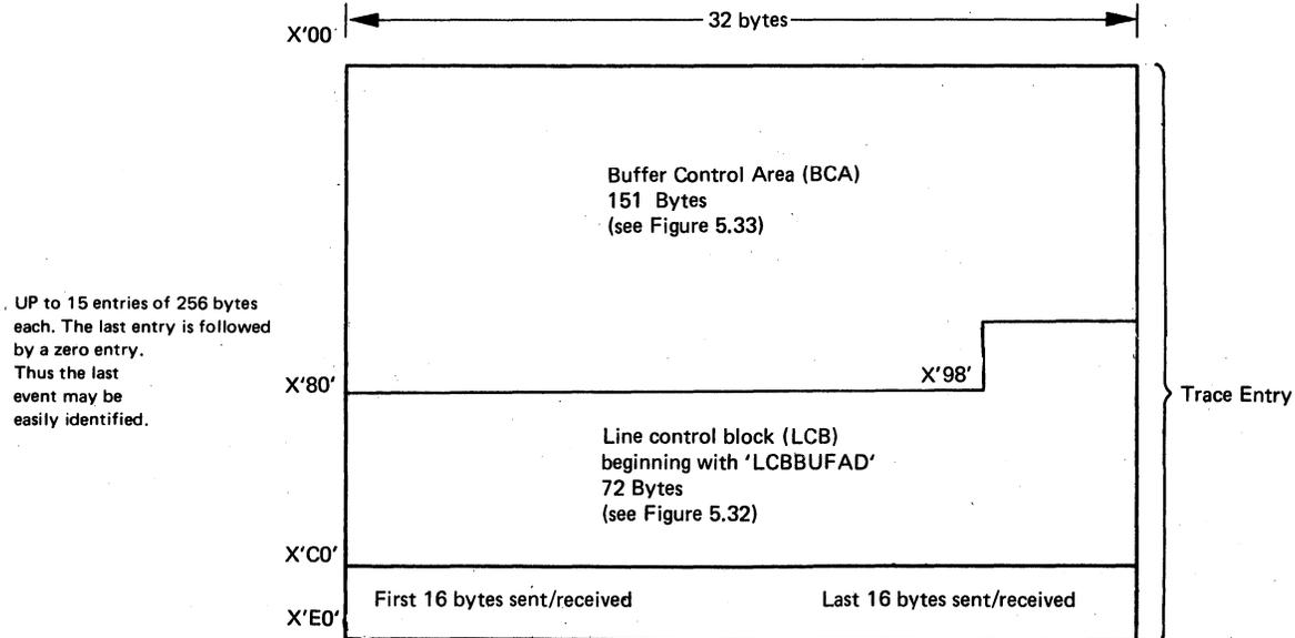
The trace is to be used when RJE,BSC line errors occur or incorrect output is encountered which can be caused by the I/O operation.
