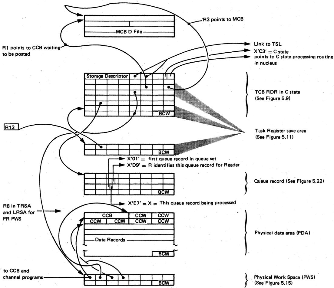
Figure 5.48. Part 5: Relations between data areas in use by task 2, showing the PWS and PDA
