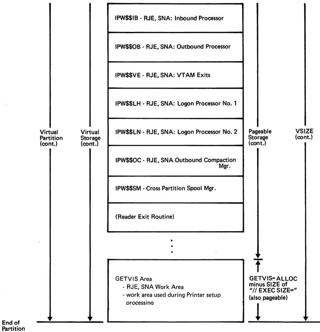
Figure 5.0. POWER/VS Partition Storage Layout (Part 4 of 4)
