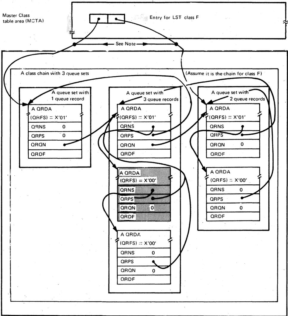
Note: All pointer addresses are seek addresses, except those in the MCTA entries, which point to queue records on the queue file relative to the MR which is record 1. (The shaded queue record corresponds to the queue record being processed as shown in part 7 of this figure).
