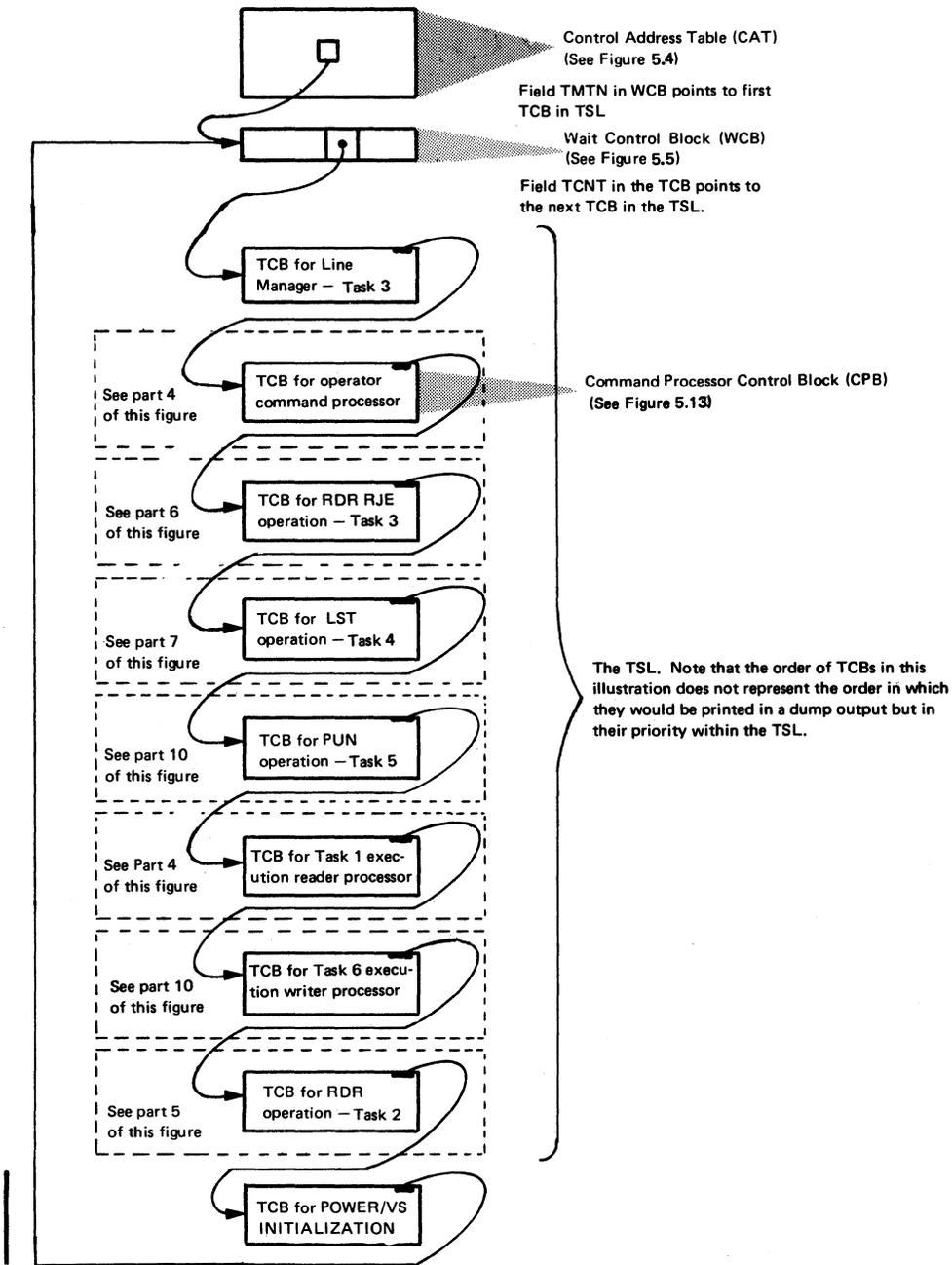
Figure 5.48. Part 2: The Task Control Blocks (TCB) linked into the Task Selection List (TSL)
