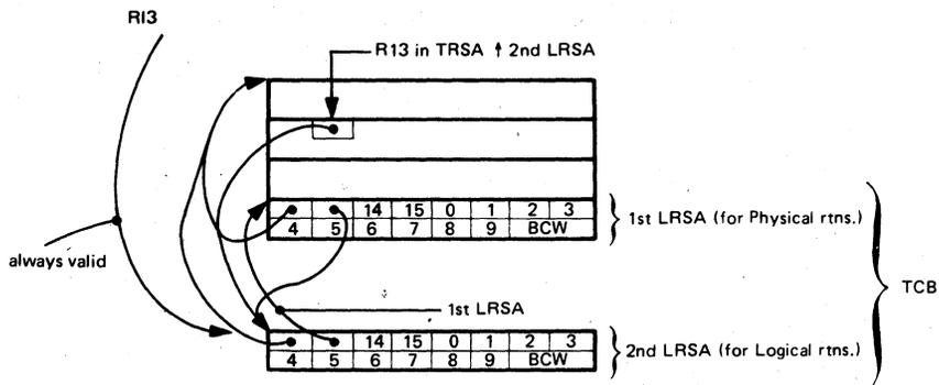
Figure 5.14. Part 2: Linkage between the two LRSAs in a Double Linkage Register Save Area (case 2)
