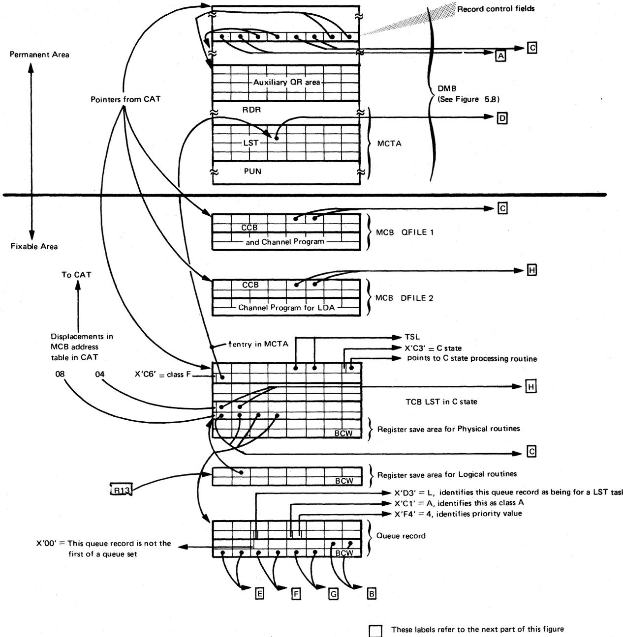
Figure 5.48. Part 7: Relations between data areas in use by task 4 showing pointers to the Queue and Data files
