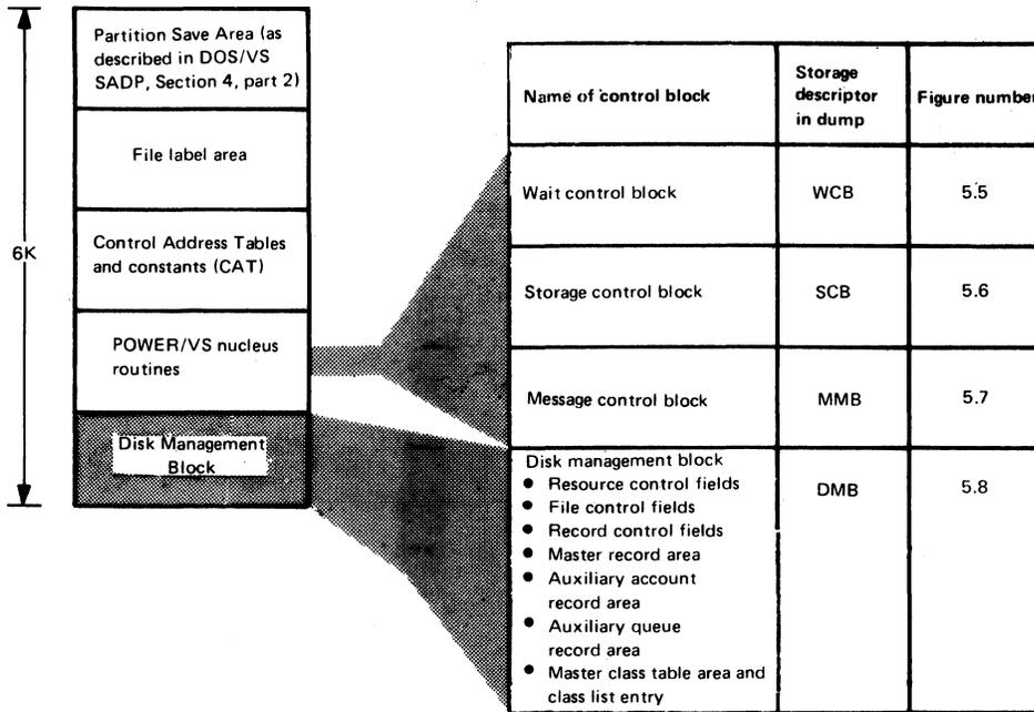
Figure 5.2. Organization of the POWER/VS Permanent Area with fixed control blocks
