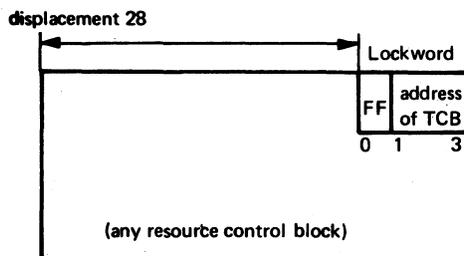
Figure 2.13. Resource lockword of a POWER/VS control block
