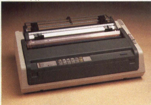
The C-line printers, Facit C5500 and Facit C7500, provide 250/400 cps, color graphics, multi-interfacing and flexible paper handling.
