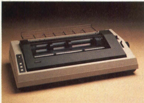
The 132-column Facit 4514 printer features NLQ as well as Epson FX and IBM PC character and command sets.
