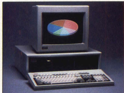
The Deskpro 386, dubbed the St. Estephe, is Compaq's early entrant into the 80386 CPU arena. It is a 32-bit workstation with a 32-bit bus and comes in two models with a color graphics option.
