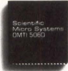
This proprietary chip transfers data as fast as the head can read the disk.
