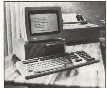
The system unit of the $2,695 DECmate III word processor, measuring 11½ inches by 11 inches by 5 inches, is DEC's smallest ever.
