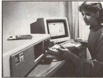
DEC's new Professional 380 workstation boasts double the performance of the earlier Pro 350, thanks to the J11 chip set.
