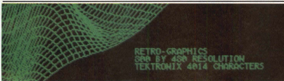
Retro-Graphics generated plot with Tek 4014's smallest characters [133 char x 64 lines] displayed at 800-by-480 bit-mapped resolution.
