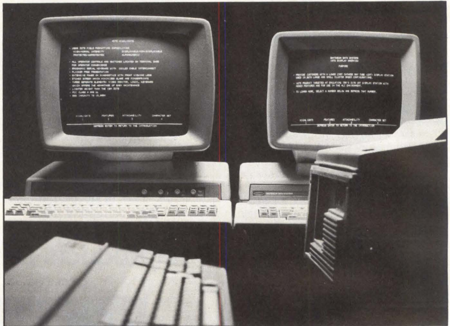
Raytheon Data Systems' PTS-1000/4000 product family includes a 12- and a 15-inch diagonal display, printers and control units that provide 3270 data-processing functions.
