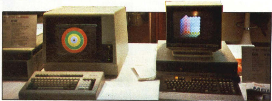
Two computers from Japan's Sord are configured around Motorola MC68000 processors. The M68 incorporates a 10-MHz MC68000. The M685 is based on the Universe computer from Charles River Data Systems, which employs a 12.5-MHz MC68000 as its CPU and a 6.25-MHz MC68000 as an I/O processor.
