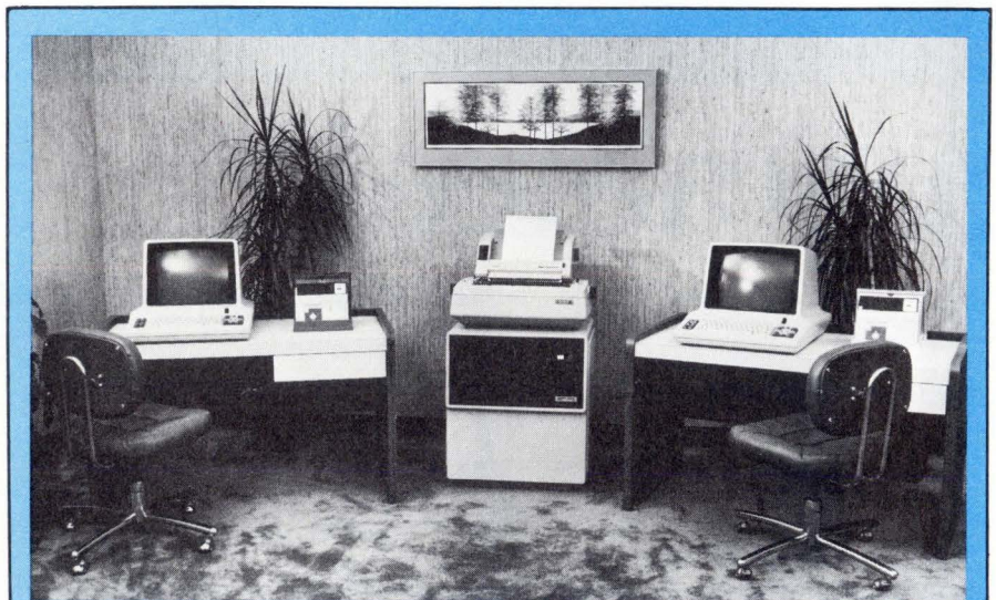
Philips Information Systems, Inc., Dallas, recently added a new member to its MICOM word-processor family—the MICOM 2002. The 2002 can be expanded from one work station and printer to four work stations and two printers. Standard storage capacity can be increased from 254 pages to more than 12,000 pages using hard disks. A base system including printer, work station and controller is priced at $13,900. The 2002 is compatible with the earlier 2000 and 2001 systems.
