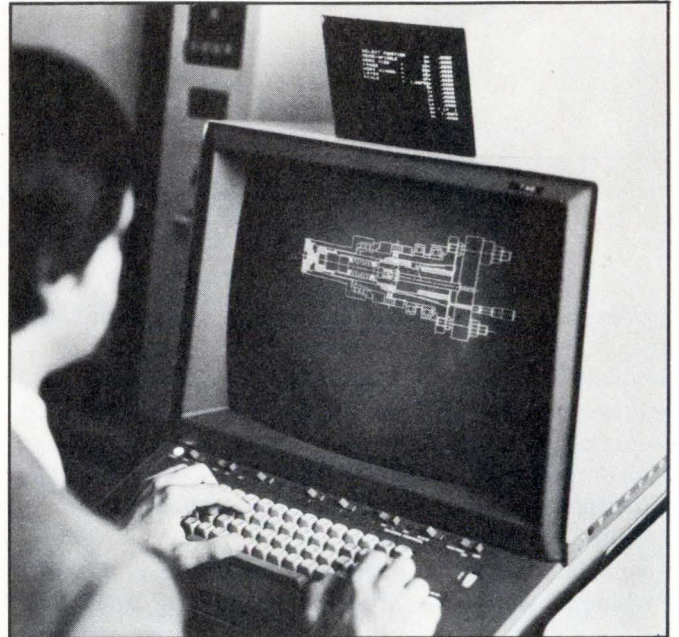
Fig. 2. McAuto's Unigraphics systems range in price from about $20,000 to $800,000 and can manage from one to 10 work stations. A total of 295 Unigraphics systems have been installed by McAuto worldwide to perform such applications as mechanical parts design and fabrication, pattern making, plastics-mold production and aluminum-extrusion die manufacturing.
