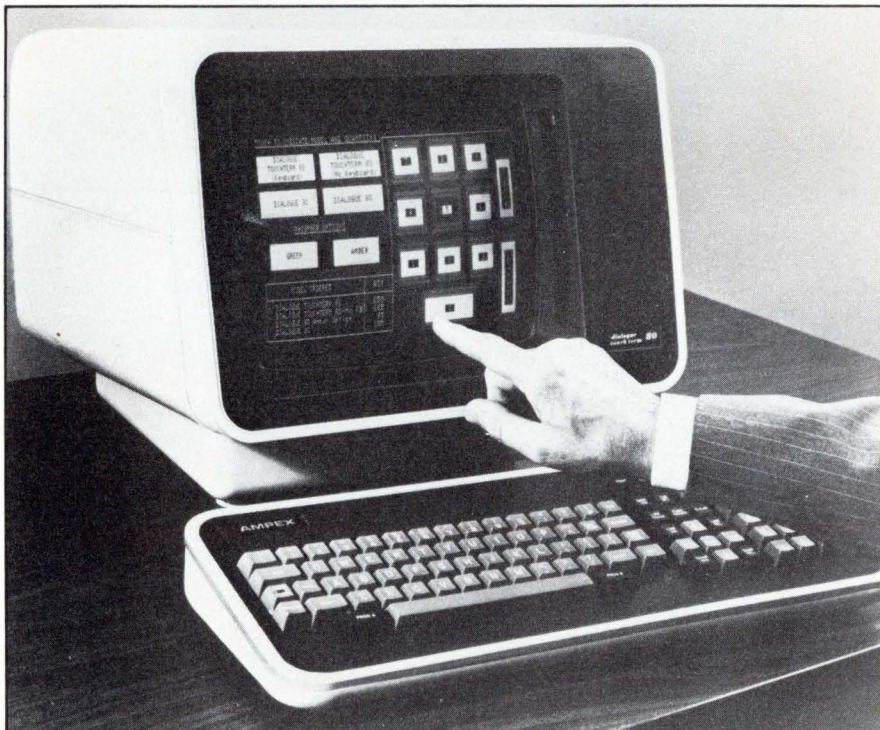
Using scanning-infrared-beam technology, Ampex's Dialogue Touchterm 80 responds to a touch on the display's terminal, thus eliminating the need for a user to have typing skills or a knowledge of special command language.
