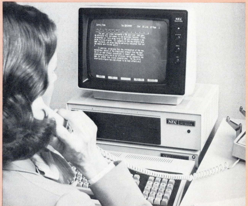
A typical PC-8000 configuration with 64K-byte RAM, 32K-byte ROM, a 320K-byte dual diskette drive, three serial communication ports operating at speeds as high as 4800 bps, a parallel printer adapter, an IEEE interface and a 2000-character CRT terminal sells for approximately $3700.
