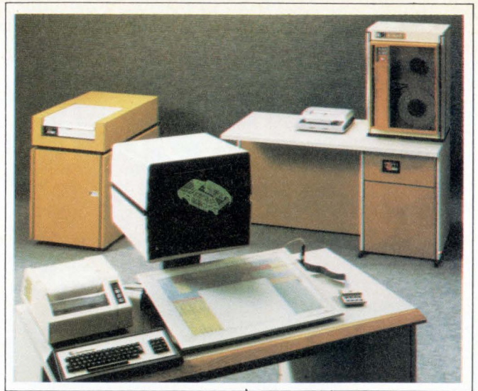
Fig. 3. The Computervision Designer system, an extremely popular turnkey CAD/CAM system, is a multi-module, hardware/software package that exemplifies the custom-configuration concept. Expandable from single-user, single-application systems to multi-terminal, multi-application systems able to support more than 30 users. The configuration shown includes a work station consisting of color raster or storage tube display, digitizer, keyboard and printer; graphics processor; disk storage and magnetic-tape drive. Additional I/O peripherals, such as pen plotters and photoplotters, as well as a broad range of additional or alternative storage devices, are available.
