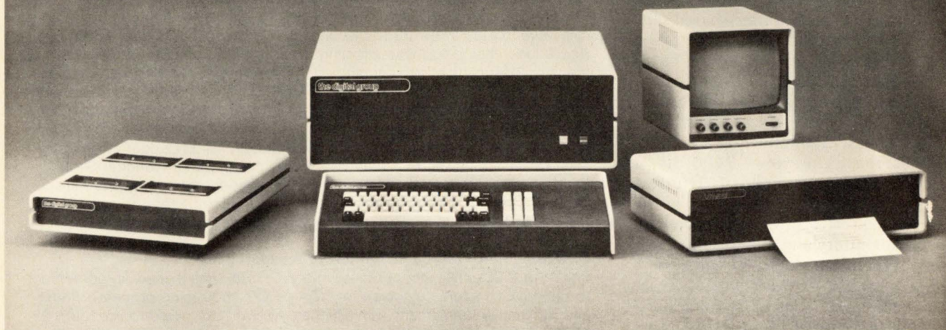
Clockwise from top: CPU, 9" Video Monitor, Impact Printer, Keyboard, Cassette Storage System with Four Drives.
