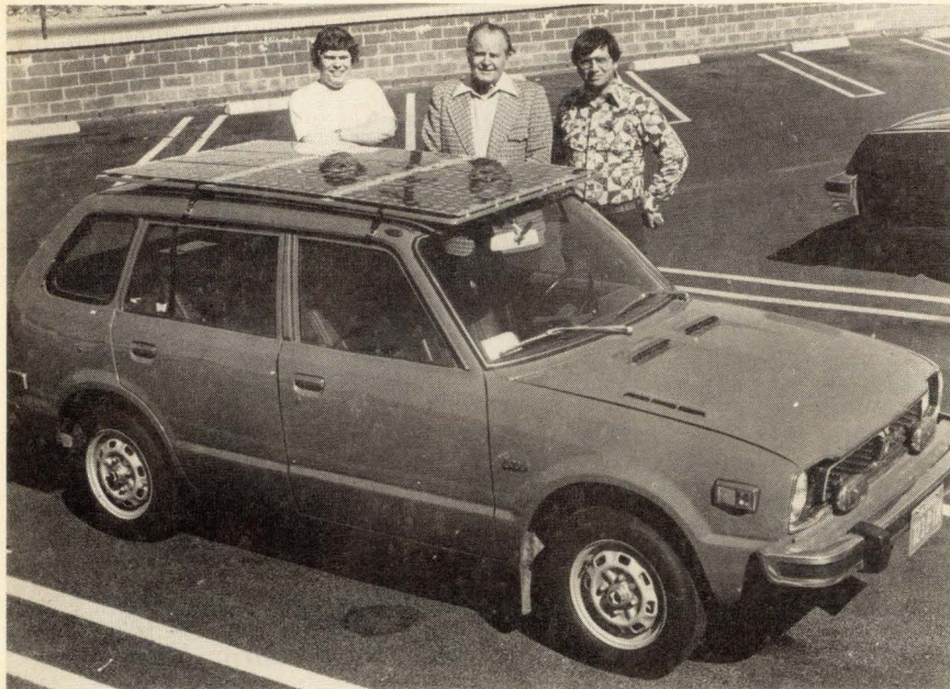
Ready for a spin. Solar-cell modules on Honda produce about 100 W for car owner Wallace C. Moore, center. Kees Van Der Pool, left, is marketing manager of module manufacturer Sensor Technology Inc. Irwin Ruben, right, is the company's president.
