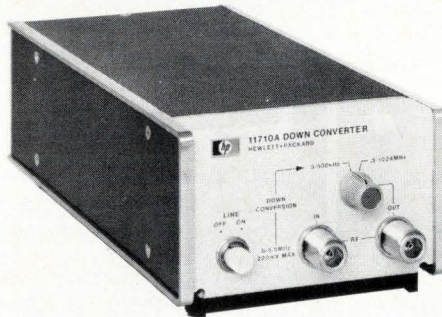
The model 11710A down converter extends the frequency range of the 8640A/B down to 5 kHz.
