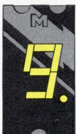
MAN 81 Common Anode; Right Hand Decimal
