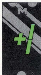
MAN 53 Common Anode; Overflow ( \pm 1 )
