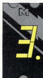
MAN 84 Common Cathode; Right Hand Decimal
