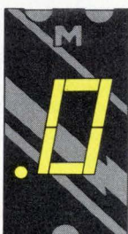
MAN 82 Common Anode; Left Hand Decimal
