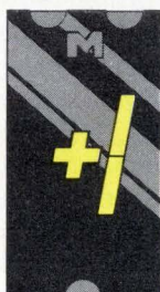
MAN 83 Common Anode; Overflow ( \pm 1 )
