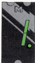
MAN 51 Common Anode; Right Hand Decimal
