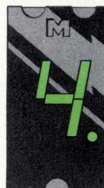
MAN 54 Common Cathode; Right Hand Decimal
