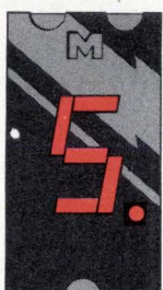
MAN 71 Common Anode; Right Hand Decimal
