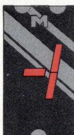
MAN 73 Common Anode; Overflow ( \pm 1 )
