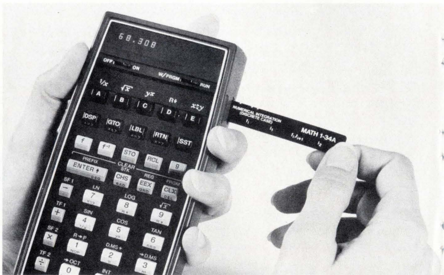
Engineer's assistant. Photo at left shows HP-65 being used to figure sidewall capacitance; right photo demonstrates method in which the magnetic program card is inserted.
