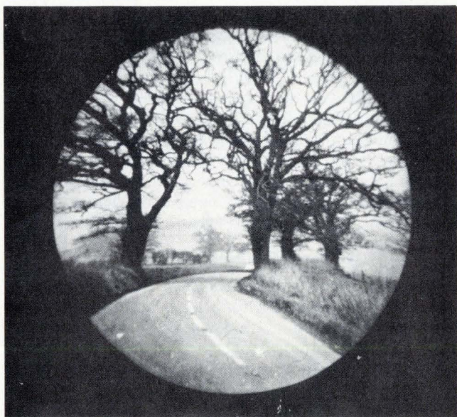
7. Bird's-eye view. Typical picture produced by microchannel-plate inverter-tube binoculars illustrates image obtainable when the tube's photocathode is illuminated at an intensity of about 3 lux (about one-quarter moon). Pin-cushion effect of inverter tube has been reduced by objective lenses with compensating barrel-type distortion.
