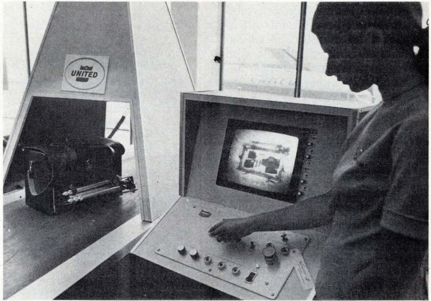
Baggage scanner. Low level X-ray scanners for inspecting baggage won't fog film.
