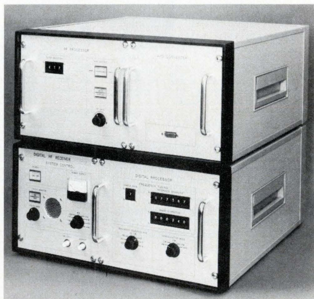
1. Digital receiver. Experimental radio uses sampling and digital filtering techniques to permit signal processing for optimum tuning.
