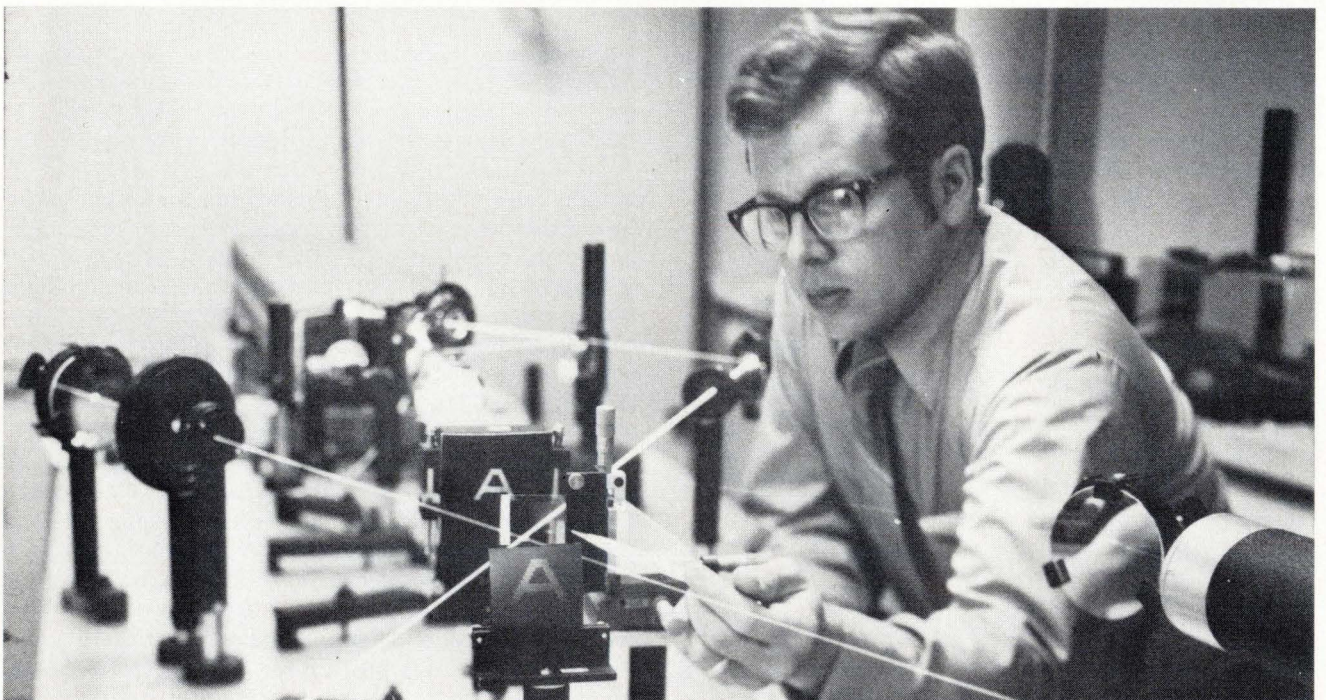
9. Real time. In a technique developed by RCA, a hologram can be developed instantaneously. A green laser is used to expose the hologram, while a red beam is used to read it out. In the setup here, the operator turns off the green beam when he has right exposure.
