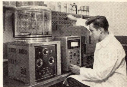
Volume and surface resistivity testing of copper-clad laminates. Exterior control unit, designed by Norplex, gives fast, reliable readout.
