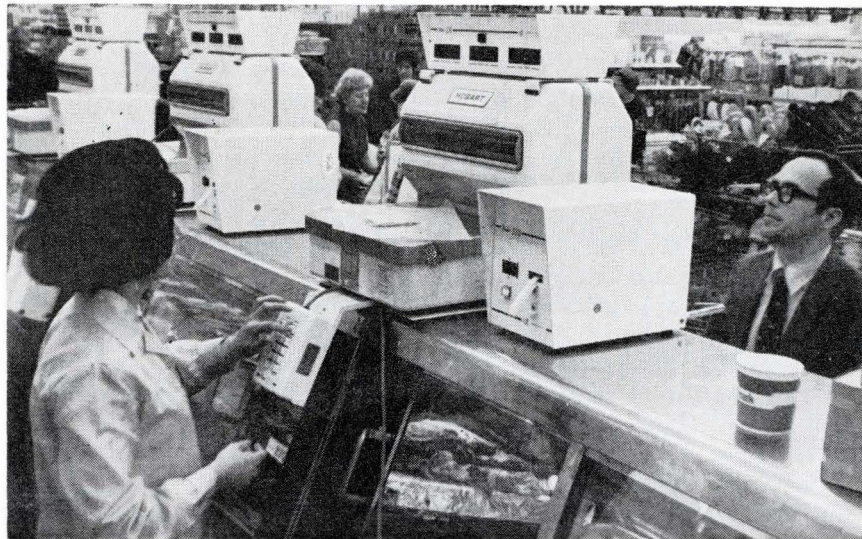
Weighing game. Retrofitted system adds readout to scale, and provides accurate weight, price information on printed label.
