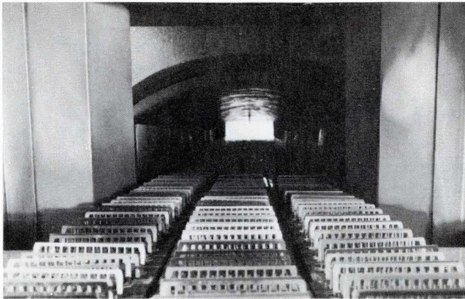
Sealing cerdip at 550° C
