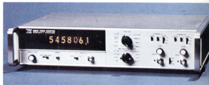
6. At work. Above, a 550-MHz binary and 400 MHz divide-by-5 quinary mounted in printed circuits to perform a decade function. Below, the packaged instrument, with frequency ranges of 0-50 MHz and 0-550 MHz.
