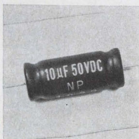
Nonpolarized, aluminum electrolytic capacitors type TNPW have welded connections joining the risers and external leads to assure a low dissipation factor and freedom from intermittent or open circuits. They offer a complete range of capacitance values from 1 to 100 \mu f and are available in voltages of 25, 35 or 50 v. International Electronics Corp., Melville, L.I., N.Y. 11746 [346]
