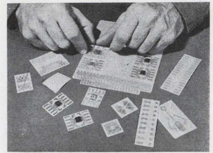
Design task. Conductive paths, then components are attached to p-c board to form circuit.
