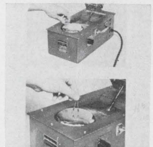
Oxide-free soldering system called Wavedipper is offered to manufacturers for a free 30-day trial. It uses a pump that continuously circulates molten solder over the reservoir lip through a circular nozzle providing a mirror-like 4-in. diameter dipping surface. The solder pot provides a cross-free application surface. Price is $750. Electrovert Inc., Mount Vernon, N.Y. [428]
