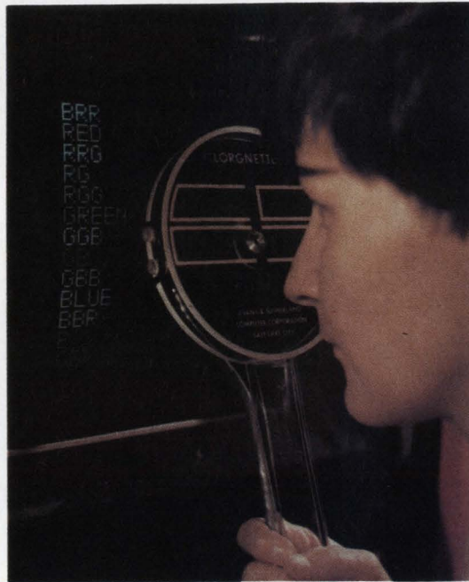
Bringing out the colors. The lorgnette at left contains the color disk, shown stationary. When it rotates, center photo, it permits the viewer to see programmed color in the computer-produced display, as at right. Another disk separates right- and left-eye images to produce black-and-white 3-D; and a third combines color and 3-D.
