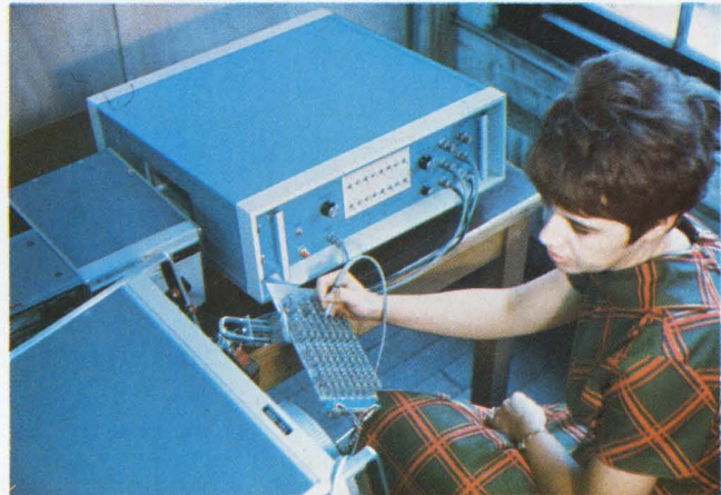
Fast and sharp. Coax cable, visible at left, preserves sharp pulses of data generator's super-speed logic.
