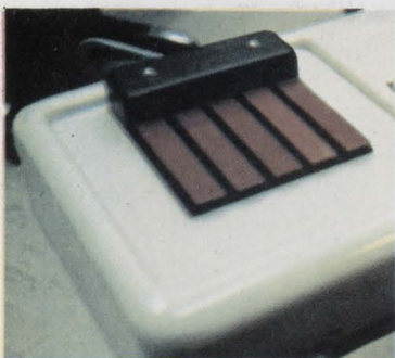
Piano keys. A binary keyboard requires tricky cross-fingerings, but allows the user to write words and codes without taking his eyes off the console or his other hand off the "mouse." With a little practice, anyone can learn to fly the system.
