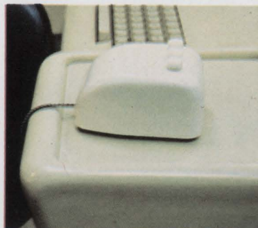
Roarless mouse. By rolling the little white "mouse" on a small, flat platform next to the keyboard, the user moves a small white pointer that appears as a spot on the cathode-ray tube display. Buttons insert words and make them disappear, and facilitate editing.
