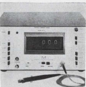
Digital current meter 801 precisely measures and displays in digital form the peak magnitude of pulse currents in the range of less than 10 ma to over 1,000 ma. Basic input sensitivity is 1 mv/ma, input impedance is 1,000 ohms and bandwidth is 50 Mhz minimum. Input pulse is 7 nec min. at the 90% points. Scientific Measurement Systems, Moorestown, N.J. [3651]
