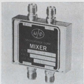
Balanced mixers series 2000 cover the frequency range from 1 to 12.4 Ghz with 15% bandwidth. Noise figures vary between 7 and 9.5 db with isolation typically 10 db. The mixers use beam-lead Schottky-barrier-type diodes, welded into the circuit and passivated. Size is 1.50 x 1.25 x 0.375 in. and weight is less than 1 oz. Microphase Corp., 35 River Rd., Cos Cob, Conn. [401]
