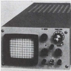
Ultracompact flexible crt display model 8602 has 11 sweep ranges selectable by a front panel control. Panel size is 3 1/2 x 5 3/4 in. with useful screen area 4 x 5 cm. Three sets of sweep ranges are available: 1 \mu sec/div. to 2 msec/div., 10 \mu sec/div. to 20 msec/div., and 100 \mu sec/div. to 200 msec/div. Infodex Inc., 7 Cherry Ave., Waterbury, Conn. 08702 [365]
