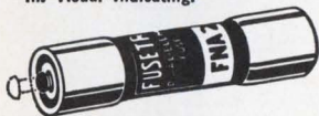
FNA FUSETRON Fuse 13/32 x 1\frac{1}{2} in. slow-blowing, Visual-Indicating, Alarm-Activating. (Also useful for protection of small motors, solenoids, transformers in machine tool industry.)
