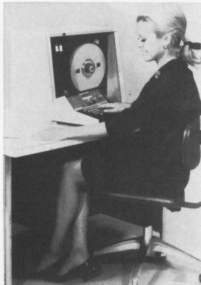
Talking to the tape. The keyboard can generate codes that have densities as high as 800 bits per inch.
