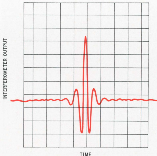
Interferogram. Output of Michelson spectrometer is a time-varying signal, this one of a broadband i-r source.
