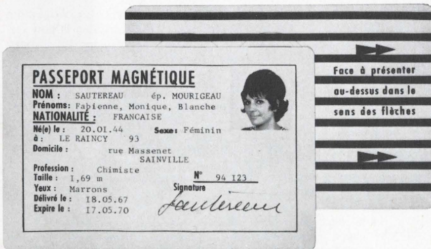
Front and back. Magnetic passport looks like ordinary ID card on one side. Data for card reader is coded onto tracks on other side.
