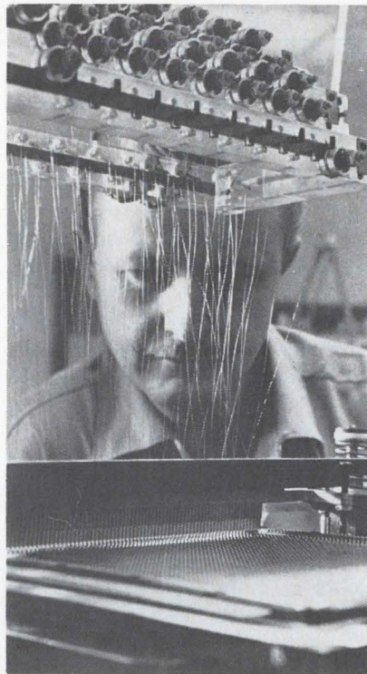
Coil weaver. Automatic machine produces interlaced twin solenoids for new rod memory.
