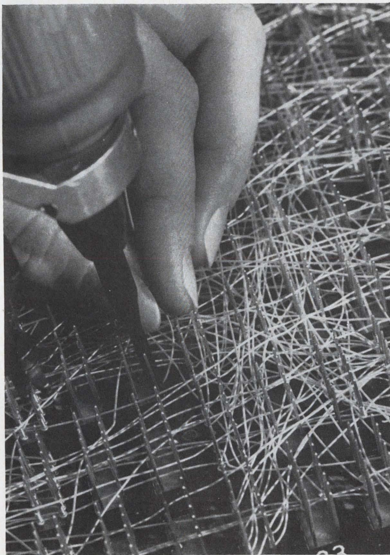
General Electric saved space and weight in wiring the back panels of its GE-PAC® Process Computers by using 30-gauge hook-up wire insulated with Kynar.
