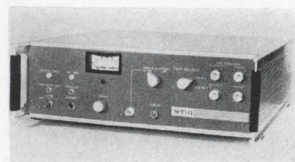
Booster. Power amplifier supplies 1 watt minimum from 1 to 12.4 Ghz.
