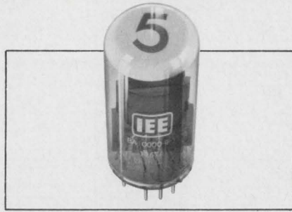
CRT Display 10-gun CRT projects single-plane digital or word displays onto fluorescent screen. Easy reading, even in direct sunlight. Wide viewing angle. Ideal for instrumentation applications.
