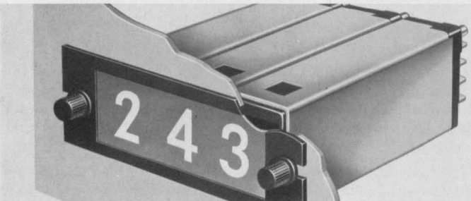
Series 875 Miniature, 24-position, rear-projection readout with .62" H x .62" W viewing area. Overall size just 1.39" H x .90" W x 3.095" D. Exceptional character brightness and clarity. Quick disconnect lamp assembly for easy replacement.
