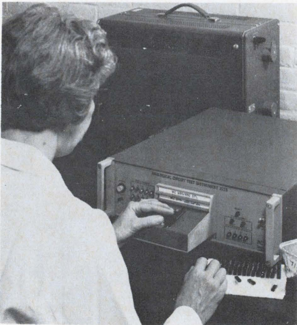
Test case. Typical, low-cost ($4,850) IC tester from Teradyne Inc. makes 15,000 analog-logic checks on digital devices in 1/100 of a second. The outlook in this segment of the market is clouded by the need to educate potential users and standardize test goals.
