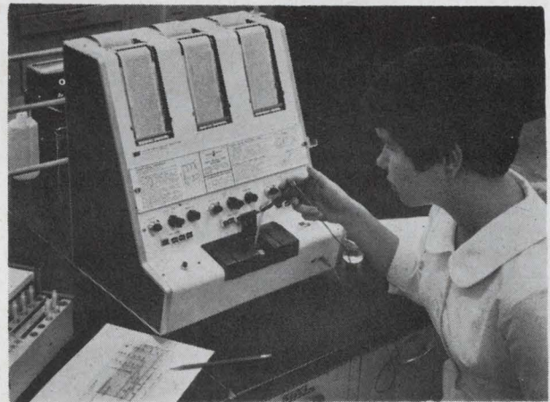
Reliable source. Electronic instruments like this coagulation analyzer from Hewlett-Packard provide better test results at less cost than conventional lab procedures; they are gaining wide acceptance.
