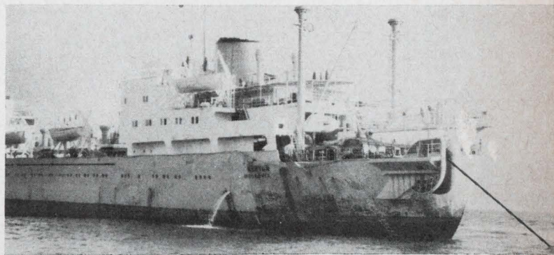
Cable ship. Neptun during the cable-laying operation. Cable is laid continuously from the front end of the ship.
