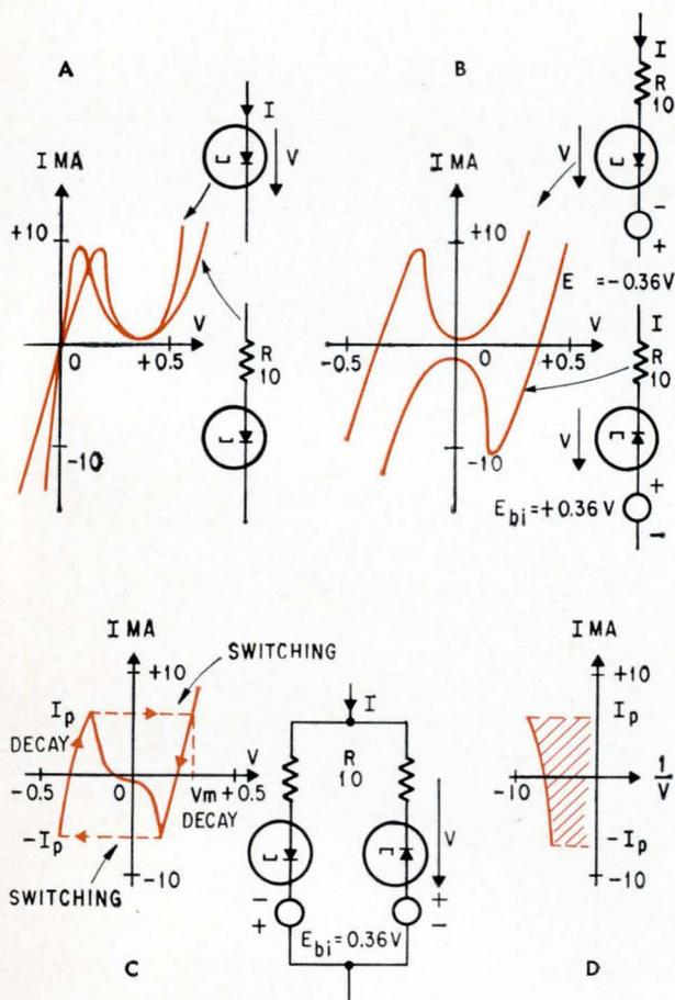
**Graphic analysis of the vco's composite characteristic** is obtained by adding the effect of the series resistance to the tunnel diode's V-I curves (A), then adding the effect of the series voltage and plotting the resulting curves for both branches on the same coordinates (B), and finally adding these curves (C). The shaded area (D) represents the integral of  $(1/V)di$  evaluated between  $-I_p$  and  $+I_p$ . This area is used to calculate the period.
