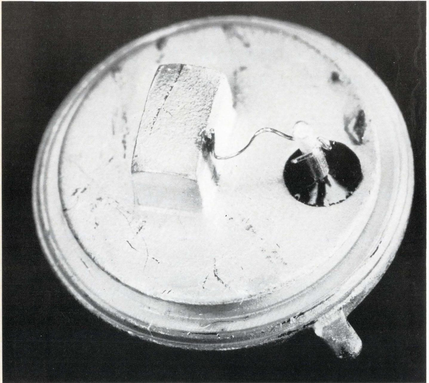
**Room-temperature GaAs injection laser** is the black speck between the wire lead and the molybdenum block. It is alloyed to a specially designed transistor header. The laser's radiation is directed perpendicular to the plane of the header.
