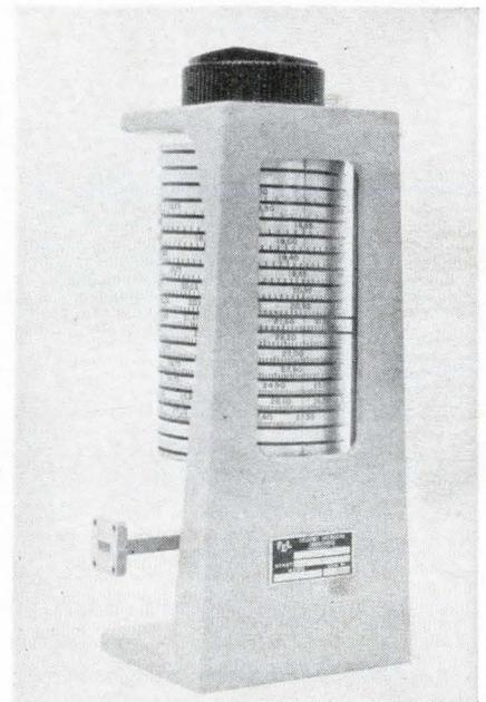
Two new precision wavemeters tune from 18 Gc to 26 Gc, and 26 Gc to 40 Gc, respectively, with an absolute accuracy of  $\pm 0.05\%$ . Because of their broad tuning range and accuracy they are especially suited for use as frequency markers in conjunction with broadband sweep generators and spectrum analyzers, or in calibrating the frequency of a transmitter, receiver, local oscillator or signal generator.
