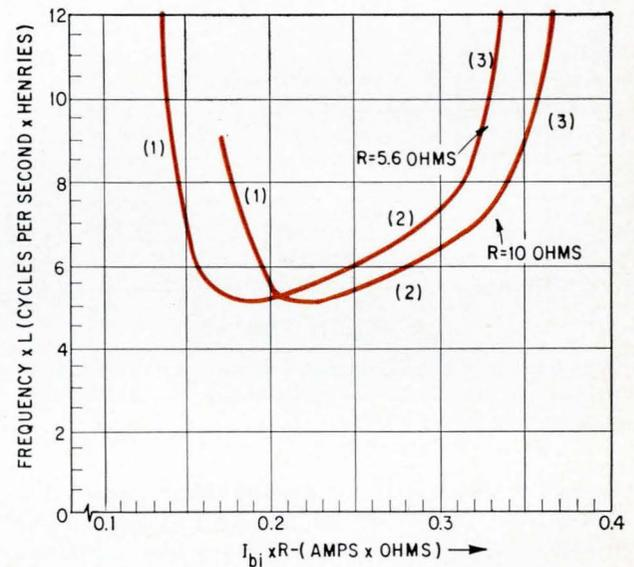
vco's frequency characteristics, as calculated from the graphic analysis, consists of three regions. Of these, region 3 is the most useful because it has a frequency swing of about  $\pm 15$  Mc about a 70-Mc center frequency, and sensitivities of 7.3 Mc/ma for  $R = 5.6$  ohms and 10.4 Mc/ma for  $R = 10$  ohms. Region 2 has a frequency swing of only  $\pm 10$  Mc and region 1 is not generally useful because quiescent  $I_{bi}$  requires critical adjustment.
