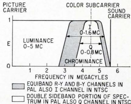
**Frequency spectrum for 625-line television used in Europe shows overlapping I and Q channels that are still used in NTSC but eliminated from PAL color-tv system. New PAL has equiband R—Y and B—Y channels.**
