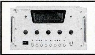
The DEI Bit Error Rate Monitor provides a means of comparing two serial NRZ data bit streams on a bit by bit basis. It accumulates the number of negative or positive comparisons over a bit interval selectable  $10^3$  to  $10^7$  bits or on a continuous basis. Provision is made for processing code forms other than NRZ. The number of bit errors (or bit matches) are presented on a visual digital display while simultaneously presented in BCD form as a printer output.
