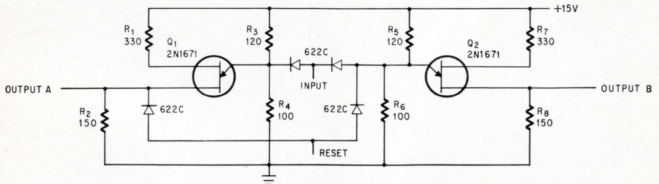
**Trinary logic element** uses two inexpensive unijunction transistors to store information in three different states. Because unijunction transistors can be constructed from a bar of silicon, the trinary module may be easily converted into an integrated circuit.
