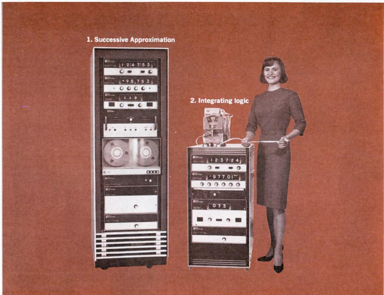
"Extensions" extend systems capabilities. In addition to a choice of logics, E-I systems offer a variety of extensions including AC voltage, resistance, pre-amp, transducer signal conditioning, thermocouple reference junctions, strain
