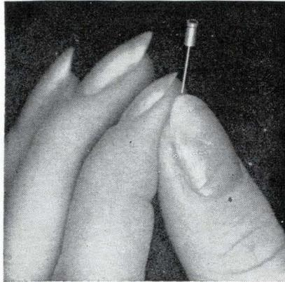
A miniature photosensor has been developed for use in tape and card readers, optically coupled circuits, encoder-decoders, character-recognition devices and process-control applications. The silicon device features planar passivation for long-term stability.
