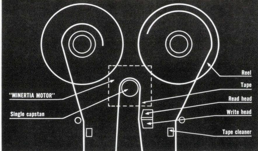
**FUJITSU ... the world's first producer of the single capstan tape handler system ... FACOM 603**
