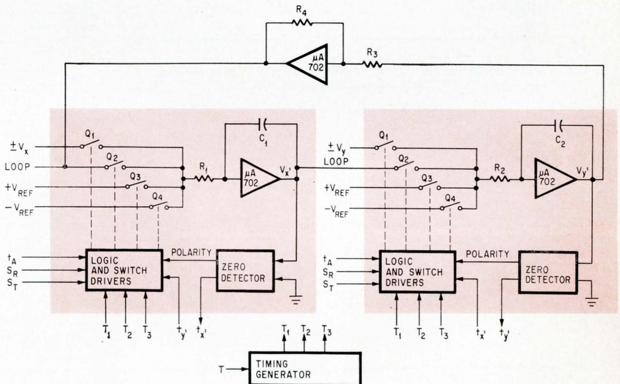
Electronic analog resolver contains two pulse-width modulators shown in color panels. Modulator at left is for  $x$  component; modulator at right is for  $y$  component. With the exception of the transistor switches, all the circuits are standard linear and digital integrated.
