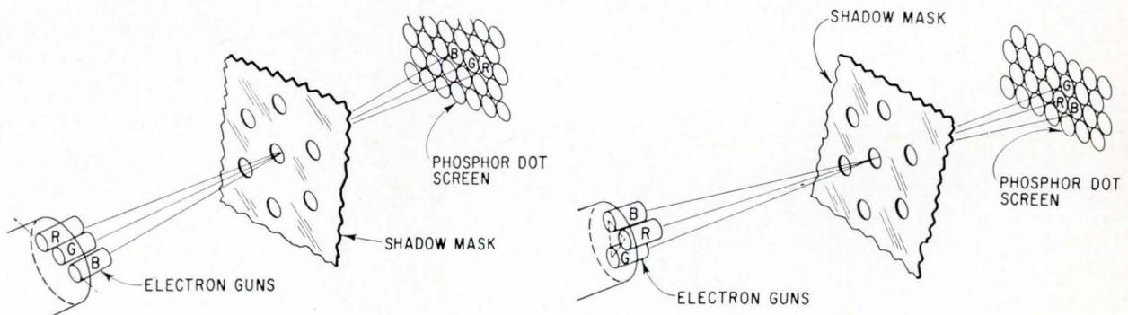
**Shadow-mask color television tube**, made by the General Electric Co., left, is similar to the conventional tube, right, except for the arrangement of the three electron guns. In the new tube, the guns are placed in a straight line; in the conventional tube, the guns are arranged in a delta configuration. With this arrangement, GE says its tube eliminates the troublesome convergence yoke.
