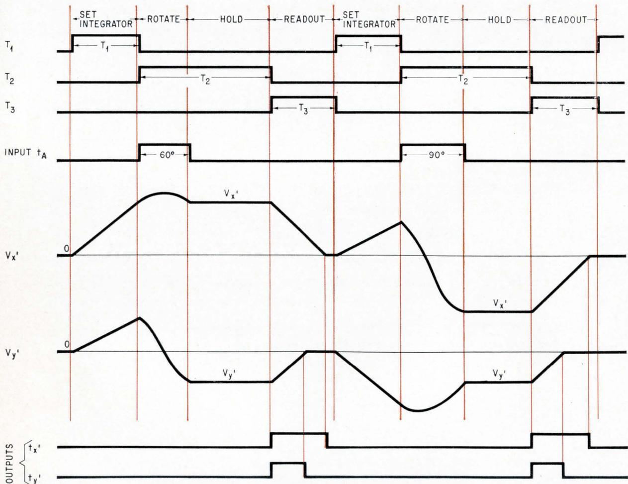
**Operational sequence** for coordinate rotation. At top are timing pulses. Representing the outputs of the integrators are  $V_{x'}$  and  $V_{y'}$ . The final coordinates are given by the width of the pulses at the bottom.
