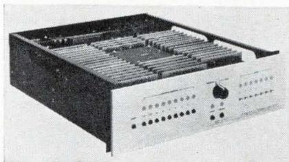
A series of magnetic core memory systems now available uses silicon monolithic integrated circuits for increased reliability. The memories have a full cycle time of 1.50 to 1.75  $\mu$ sec, with storage capacities from 128 to 8192 words for the basic unit. Access time is 600 nsec for read or read/restore operation. Date-in time as late as 800 nsec after initiation of the memory cycle speeds up computer operations.
