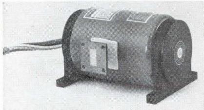
The VA-177M backward wave oscillator operates in the 10.0- to 15.5-Gc frequency range. This fully shielded, permanent-magnet-focused tube provides at least 50 mw of output power over the M-band range. Tuning is achieved by adjusting only the helix voltage. The resulting voltage-vs-frequency curve follows an exponential function and exhibits no discontinuities. A nonintercepting negative control grid provides a means for amplitude modulation without drawing current in the modulating circuit.
