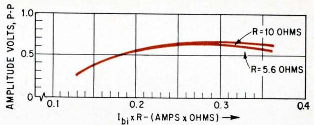
vco's output waveshape amplitude characteristics are calculated from the graphic analysis of composite characteristics obtained from different baseband input current values. The amplitude varies little over most of the range of input currents.
