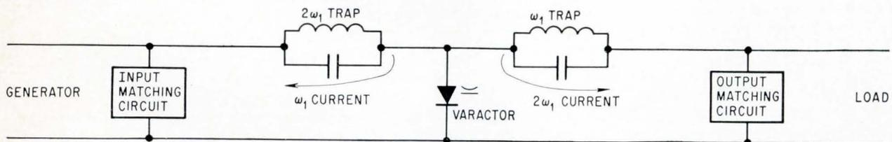
**Varactor doubler** uses traps for filtering and for matching the diode impedance. The traps are resonant at radian frequencies  $\omega_1$  and  $\omega_2$ .
