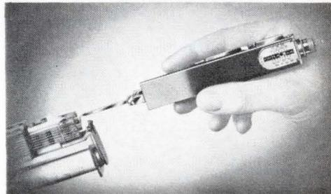
FOR checking the tension of springs or similar resistive forces.
