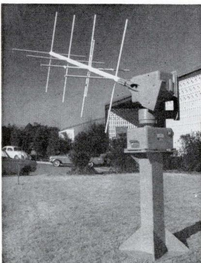
Receiving antennas of this sort, designed by Scientific-Atlanta, Inc., can pick up weather data from satellites.
