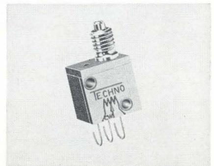
A panel mounting, miniature, square-trimming potentiometer has been developed with solder hook terminations. Model 160 features a heat dissipator as an integral part of the solder hook design. In addition, both the panel-mounting bushing and the terminating solder hooks are molded into the plastic case for rugged, dependable mechanical bonds.
