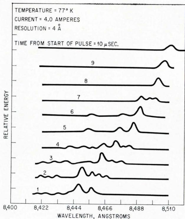
Spectra of a gallium arsenide laser are resolved in time at one microsecond intervals. When the input pulse is applied to the junction, temperature rises, causing the shift in wavelength of the radiation with time.
