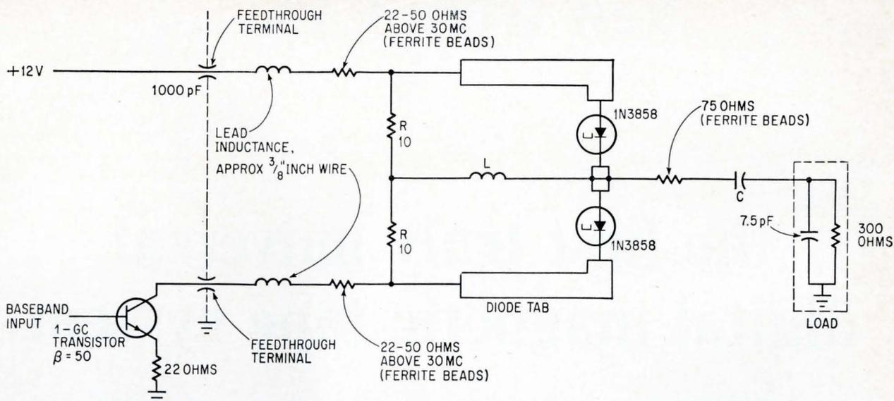
Spurious oscillations are suppressed in the tunnel diode vco by inserting ferrite beads in the input and output connections to reduce the Q of the inductance in the leads.
