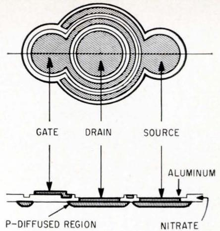
**Igfet structure.** Sketch of an insulated gate field effect transistor indicates where Sperry Rand researchers use silicon nitride for diffusion masking, p-n junction passivation, and as a dielectric.
