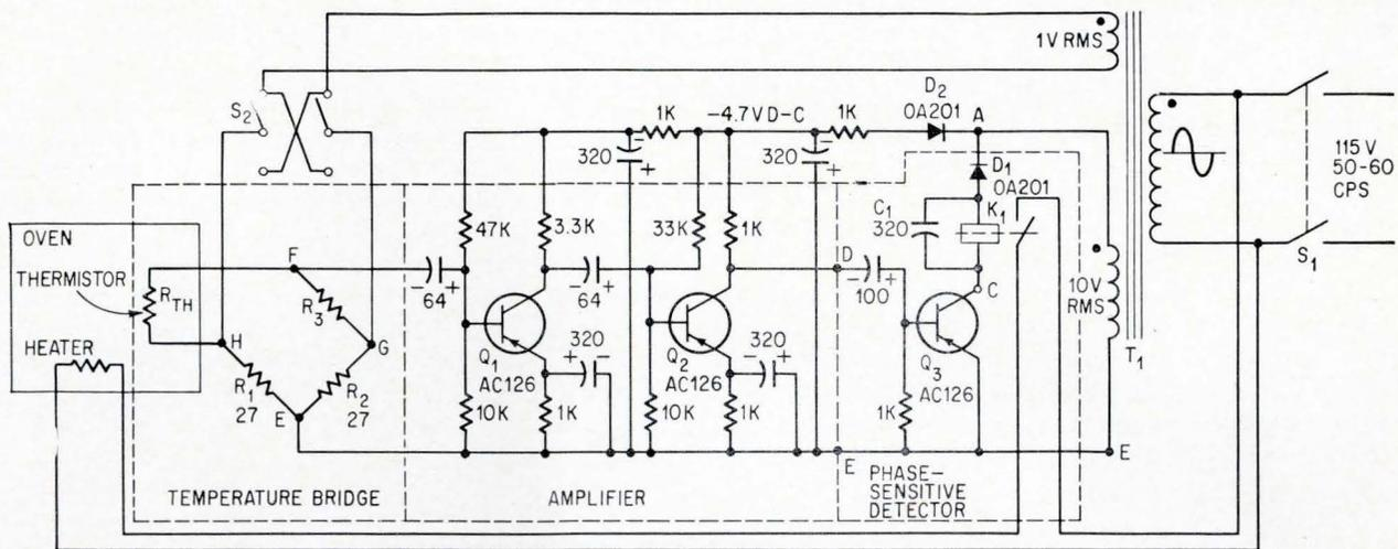
Thermostat senses an unbalanced voltage across the Wheatstone bridge terminals FE, when the resistance of the thermistor  $R_{th}$ , changes with temperature. The amplified error signal actuates a relay which controls the heater voltage.
