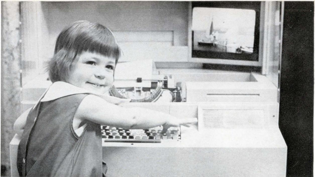
Called the **talking typewriter**, this machine, developed by the Edison Laboratory division of the McGraw-Edison Co., helped preschool children learn to read, write and touch-type. It contains computer-controlled keyboard, random-access audio storage and slide projector.
