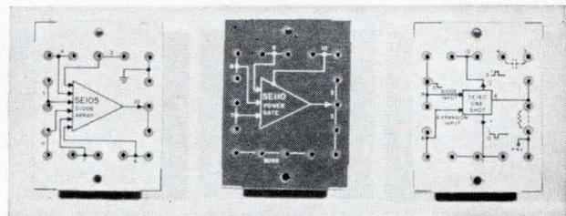
**Color-coded decals**, affixed to boards using the same printed circuit, differentiate the various logic functions. The decals also indicate the interconnection terminals and the discrete components mounted on the boards.
