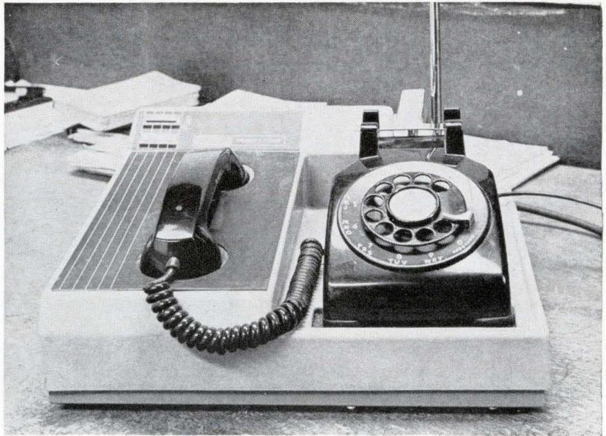
**Telephone cradle** contains equipment to receive outside calls and relay them to an eight-ounce transceiver as far as a half-mile away. The system, developed by the Chromalloy Corp., permits two-way conversations.
