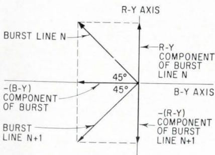
**Color phasor diagram** shows direction of proposed color burst for lines n and n+1. Alternating position of the burst simplifies receiver design.
