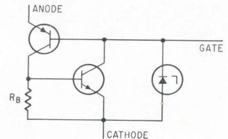
**The silicon unilateral switch, developed by the General Electric Co., has a lower breakover voltage than most diodes.**
