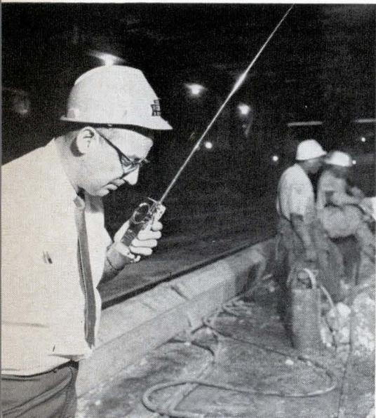
**Pocket-size "extension phone"** handles telephone calls even though the user is out of the office.
