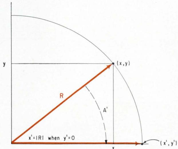
Trigonometric operations which rotate coordinates through an angle  $A$  (top) and transform coordinates from rectangular to polar form (bottom).
