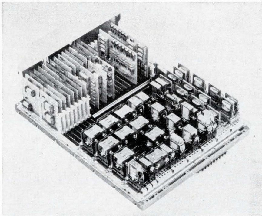
A complete line of hardware that can be used for packaging electronic circuits, subsystems and systems is being offered by the International Business Machines Corp. The line, called SMS for standard modular systems, has been used by IBM in over 15,000 computer installations since 1959.
