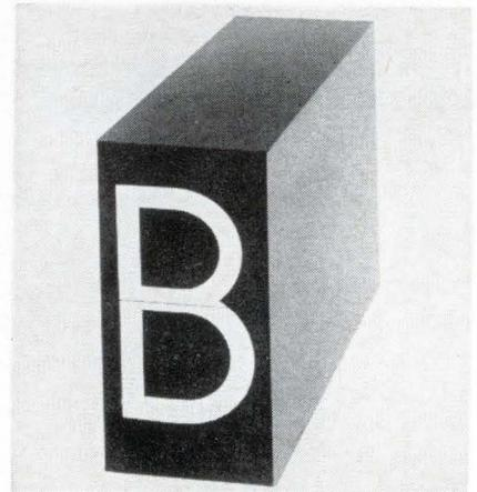
The 404 alphanumeric, 40-position readout uses the new flap principle to display numbers 0-9, alphabet A through Z, 4 in. high and 2 in. wide, with four blank positions that can be used for display of special symbols. Readout characters are of high-contrast white on nonglare black, with unlimited color combination selection optional. Display definition remains constant regardless of ambient light conditions. No bulbs or luminous or projection devices are used.
