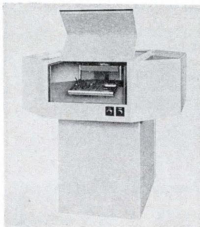
Model 562 is a fully automatic solder coating system that uses centrifugal force to leave a smooth, even solder coating on printed circuit boards. It meets MSFC 154.
