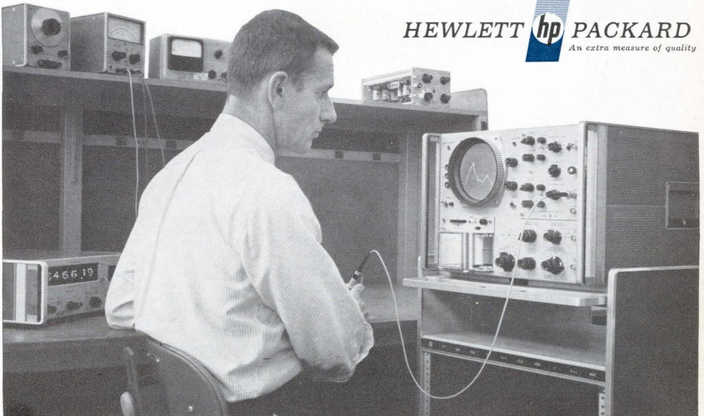
The 175A Scope, 1755A Vertical Amplifier Plug-in and 1781B Sweep Delay Generator give you the exclusive 20 and 50 MHz dual-channel performance listed above—for only \$2225!
