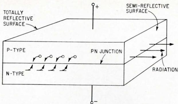
**Forward-biased gallium arsenide laser diode.** Holes from the p semiconductor material and electrons from the n material are injected into the space-charge region on either side of the junction. Upon recombination of the carriers, radiation is emitted from the diode.
