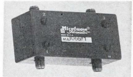
An ultraminiature, 4-port, ferrite circulator has been developed for X-band. The MA-3066 operates in the 8.5- to 9.6-Gc frequency range with less than 0.25-db insertion loss between ports 1 and 2. Maximum vswr is 1.2:1 with isolation of 20 and 40 db between ports 2 and 1, 3 and 1. The compact unit uses OSM connectors and weighs less than 4 oz.
