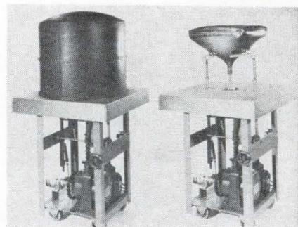
A high-vacuum cart now available is designed to exhaust color and black-and-white tv tubes, and can be made to the dimensional specifications of the customer. It consists basically of a water-cooled header, a 1½-in. low backstreaming water-cooled diffusion pump with solenoid-actuated, quick-quench boiler coil, and a Hyvac 14, two-stage mechanical forepump with water-cooled baffle.
