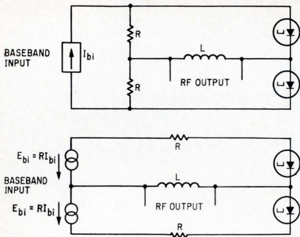
**Basic circuit** of a tunnel-diode oscillator with constant-current drive, top, and its equivalent circuit, bottom. The circuit oscillates because the tunnel diodes alternately switch between their high- and low-voltage regions.
