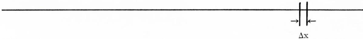
$\frac{\Delta x}{\Delta i}$  on a flat face CRT increases center to edge
