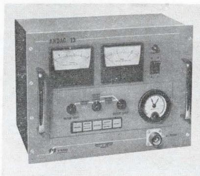
A new circuitry development, which supplies a completely static constant current battery discharge, is utilized in this battery charge-discharge capacity analyzer. The battery analyzer, discharger, and charger, designated ANDAC, provides complete and automatic electrical check-out of such exotic batteries as silver-zinc, silver-cadmium and nickel-cadmium, as well as conventional lead-acid batteries and individual cells of any battery type.
