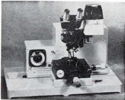
A mechanical alignment and inspection machine for integrated circuits is designed specifically for the semiconductor integrated circuit industry. Model 702 is both a work station for the precise alignment of a glass mask with patterns on a semiconductor wafer, and an inspection station for masks and wafers.
