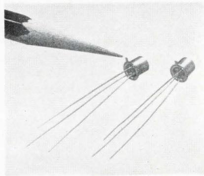
**Inexpensive monolithic** integrated circuits that do the job usually done by four-layer diodes have been developed by the General Electric Co. The devices have lower breakover voltages than most diodes, and are temperature-stabilized.
