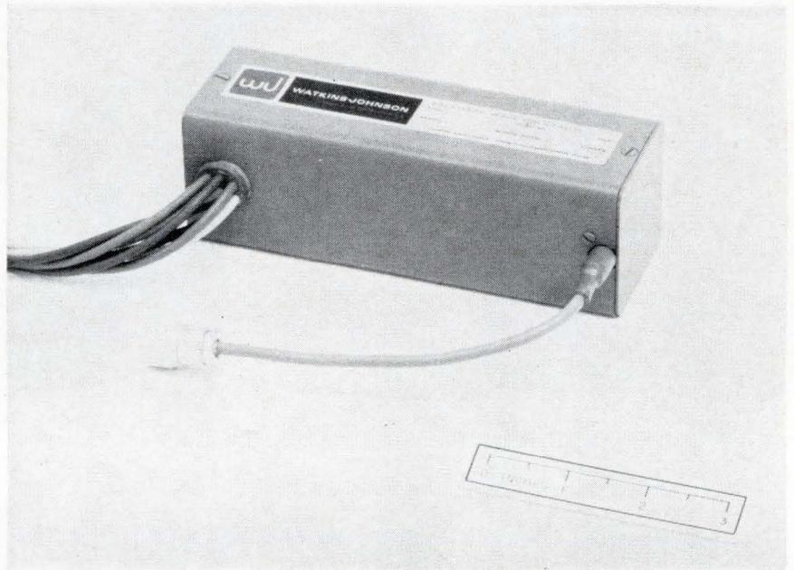
**Microwave tube oscillators** for airborne and missile applications must be small and light as well as rugged and reliable. The size and weight of these tubes is primarily determined by the magnet structure accompanying the tube for focusing the electron beam.
