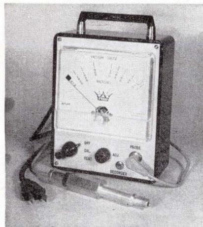
The Thermivac vacuum gauge uses matched thermistors to measure vacuum in the 2,500-micron to 1-micron range with accuracy to 1% of full-scale deflection. A built-in jack for recording the 1,000-mv signal is provided.
