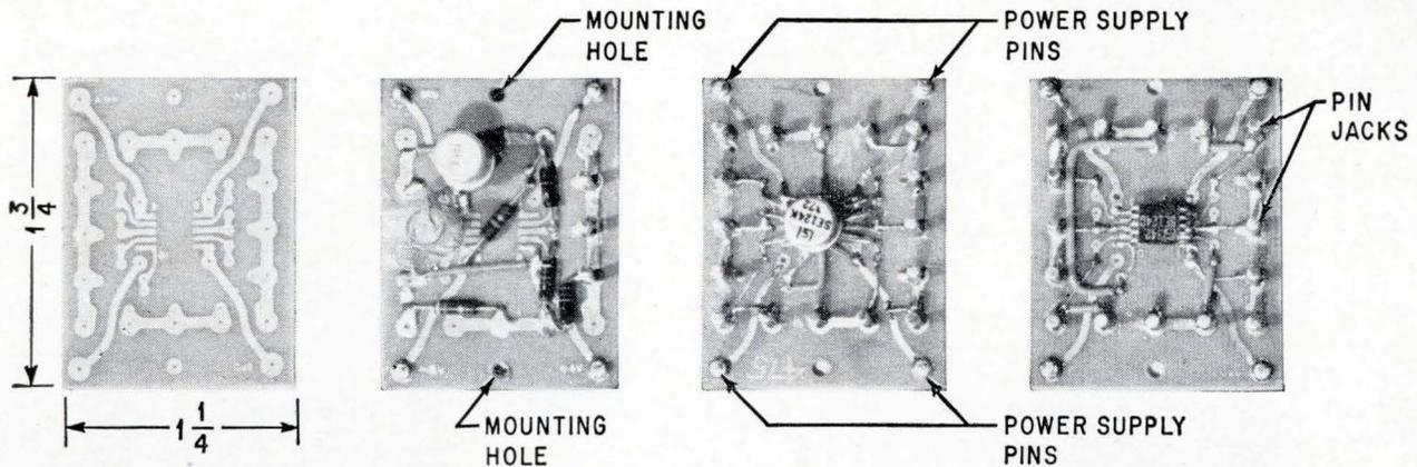
**Modules** are supplied with mounting holes for inserting a thumb-screw that engages a threaded hole on the mounting strips. Terminals are miniature pin jacks which accept pin plugs for interconnecting the modules. In each of the four corners is a pin for a pressure connection to the power-supply strips.
