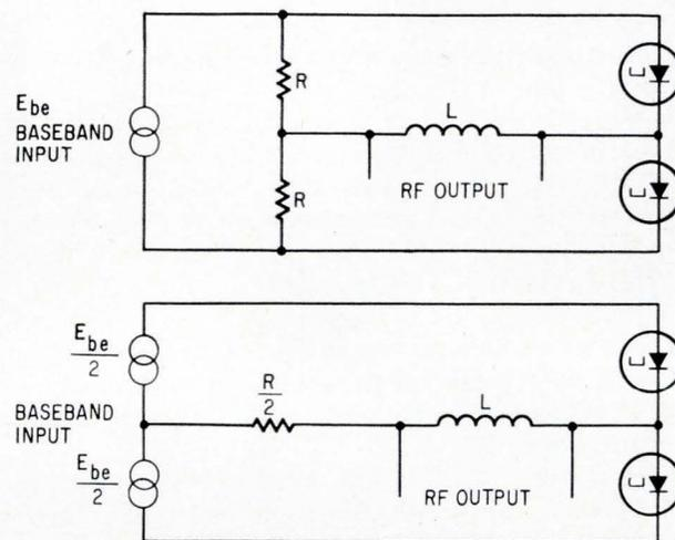
**Constant-voltage** drive provides better linearity in region 3 than constant-current drive, although it may be difficult to build the circuit because of the vco's low input impedance. The actual circuit, top, can also be analyzed graphically using its equivalent circuit, bottom.
