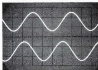
Phase lock; output from function generator (upper trace) locked to external fundamental (lower trace).
