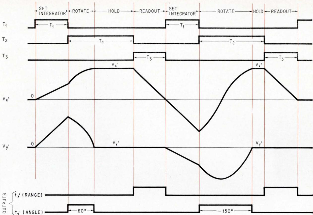
Operational sequence for coordinate transformation. Note that one of the output pulses starts at  $T_2$ , the other at  $T_3$ .
