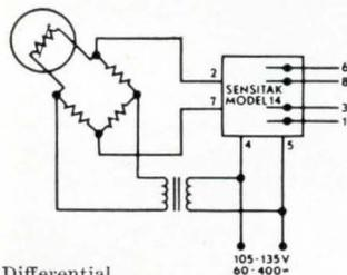
Differential Thermistor (temperature controller)
