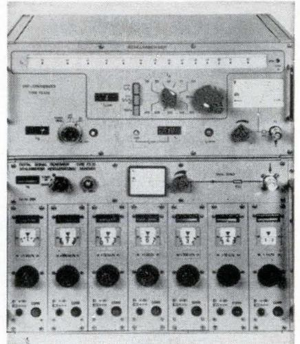
Two solid-state frequency synthesizers are being produced by Schlumberger Overseas GmbH, of Munich, West Germany.
