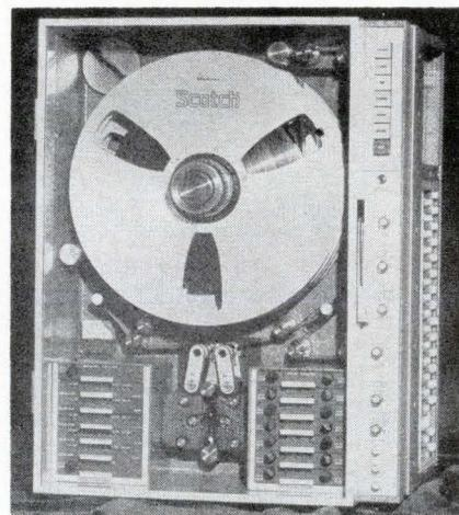
The latest model in the PC-500 portable coaxial recorder series extends its wideband capability to seven or fourteen 2-Mc channels at 120 ips, with two selectable reproduce-monitor tracks. The system is contained in a 4-cu ft package only 24 in. high. It accommodates 10½-, 12½-, or 14-in. NAB standard or precision reels.
