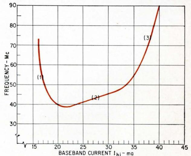
Measured frequency-baseband current characteristics. Region 3 has a 40% bandwidth with respect to 74-Mc center frequency.
