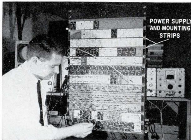
Integrated circuit packages are mounted on individual modules and are interconnected to set up a breadboard circuit. Power is supplied through a printed circuit board that is sandwiched between insulator strips mounted along the face of the rack.
