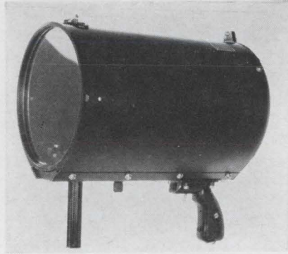
Hand-held optical communications unit converts voice signals into light pulses. Receiver reconverts the light into voice signals.
