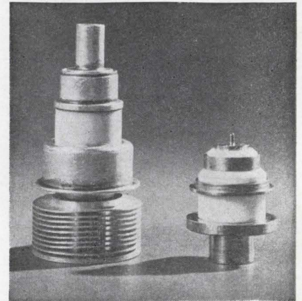
Experimental triode type L65/Y1430, right, supplies c-w power levels 20 times greater than the widely used 2C39 triode. Design improvements have also resulted in unusually high gain-bandwidth products for the L-65.
