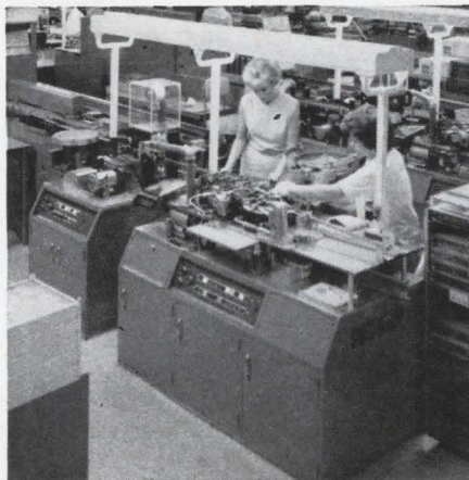
Figure 2. TI's mechanized alloy transistor assembly machine—an industry exclusive—insures uniformity and reliability at very high production rates
