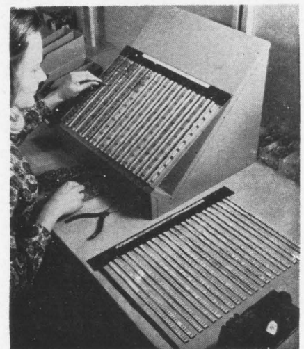
Symbols on aluminum strips indicate types of components and their location, when template is placed on terminal board
