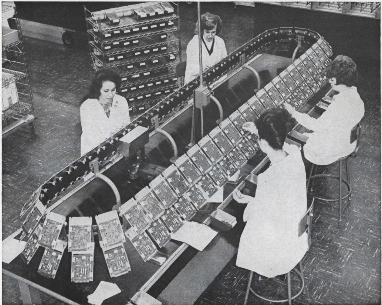
Double-decker line allows operators to work on two production runs simultaneously, or to divide tasks on one run for higher production rate.
