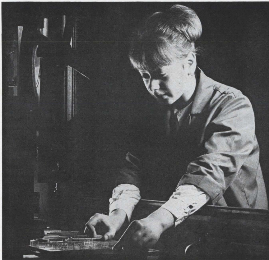
Component board is removed from numerically controlled machine at Standard Telephones and Cables' new plant in Basildon, Essex. Machine drills the boards and inserts small terminal posts.
