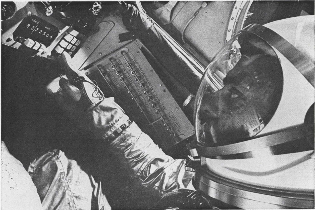
Astronaut enters data into Gemini computer, using manual data-insertion unit. Display portion of the unit appears at left of keyboard.
