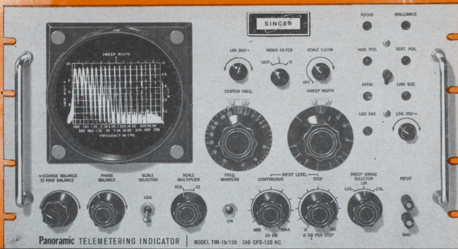
TMI-1b/120 Indicator —spectrum presentation of 18 IRIG channels showing slight preemphasis of higher channels. Log scan, log amplitude.
