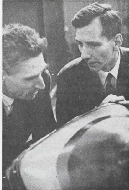
New color-tv tube is studied by CFT engineers. Dark border on tube contains electrodes that adjust electrons' speed.
