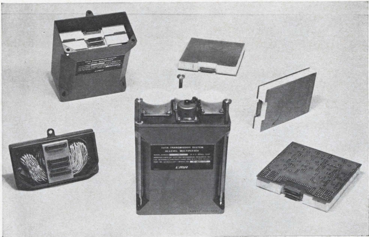
The high-level multiplexer, showing polyurethane foam encapsulant used for individual assemblies. The complete unit is at center.
