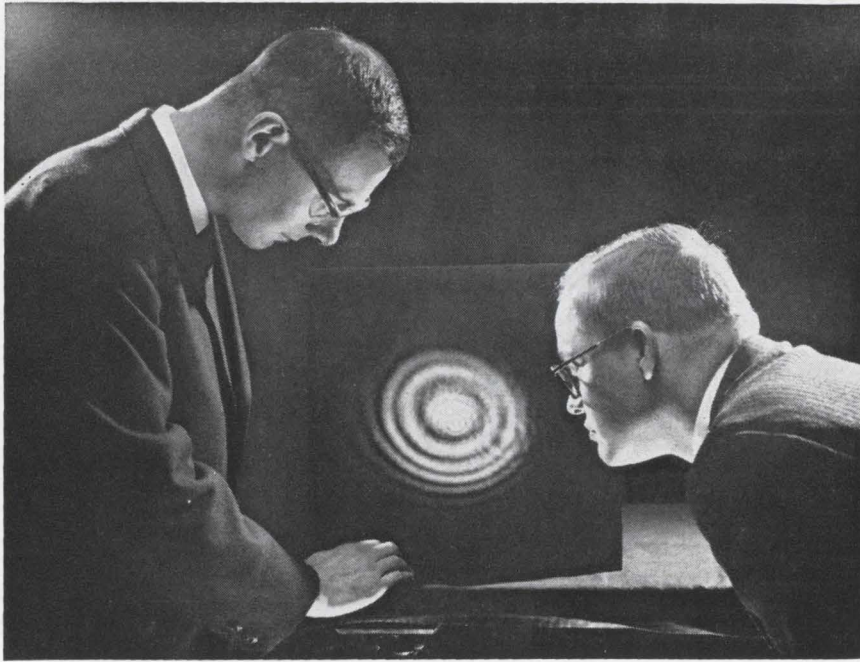
Interference rings are formed when two laser beams are at the same frequency at a constant phase difference. John Rodda, left, and Louis Enloe of Bell Telephone Laboratories developed the method of locking two beams in phase.
