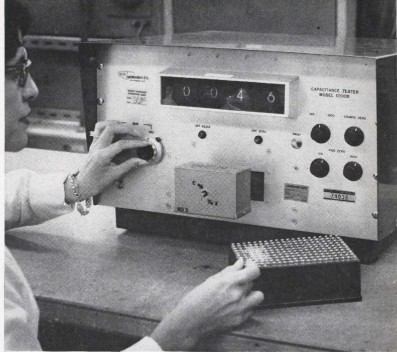
Technician checking total capacitance (can, junction and bonding island) for a 2N3493 transistor with a reverse bias of two volts. Meter reading is 0.46 picofarad 0.7 picofarads is guaranteed maximum at three volts.
