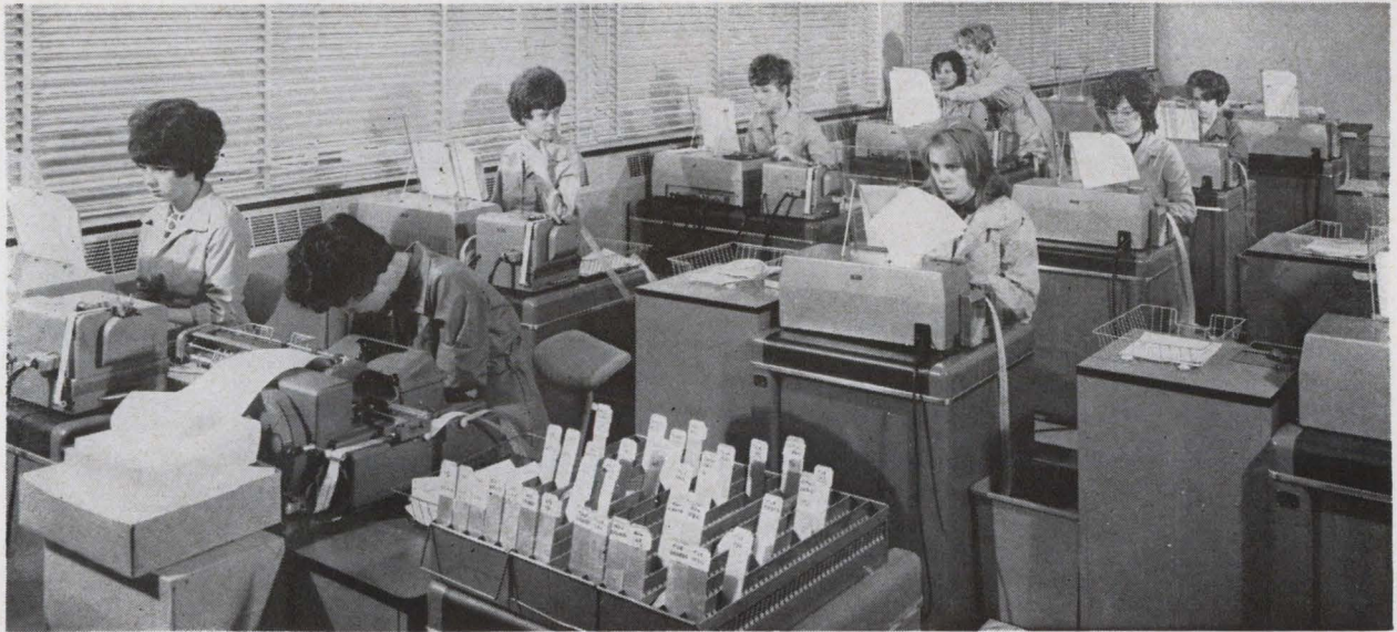
Girls punch incoming orders into tapes that are then taken next door and read into the executive computer using tape reader, right foreground, in photo at left.
