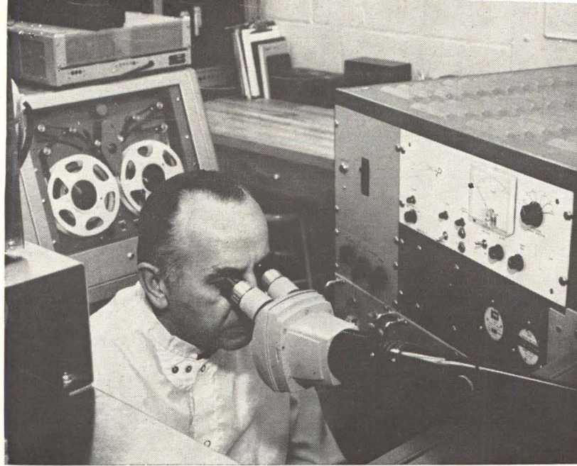
Tape-programmed electron-beam machine. Operator peering through binoculars is monitoring the operation. A wired-program machine is used to produce the two micro-modules shown. One module is a binary divider with 20 integrated circuits. The other is a sense amplifier with chip semiconductor devices and deposited thin-film resistors.
