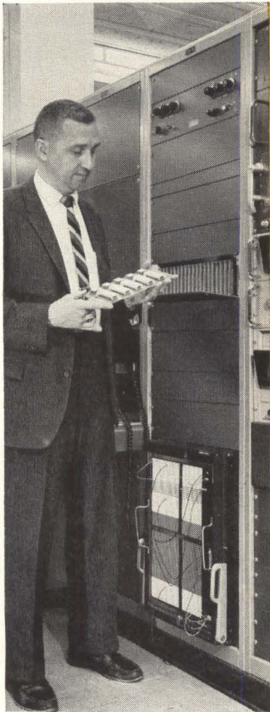
Clare Control Modules provide both high level and low level switching circuits in the NASA-Lewis Scanner system.
