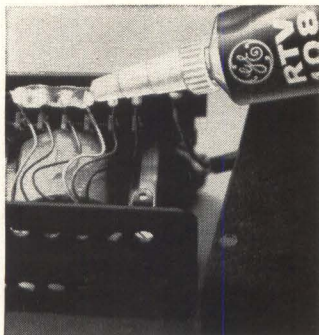
1. RTV-108 provides instant, "see-through" insulation as well as vibration resistance and environmental protection. RTV needs no pre-mixing; is applied directly from the tube.
