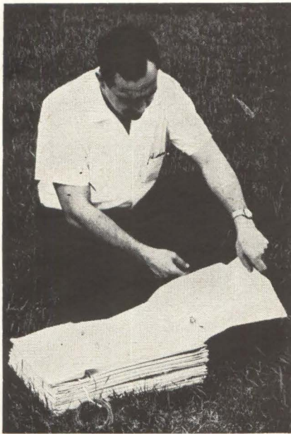
Inflatable package can become a 50-foot antenna, thereby getting over some of the foliage that blocks transmission in South Vietnam.
