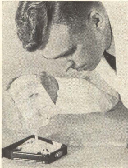
After slurry is poured into mold, it will rise like yeast bread dough.
