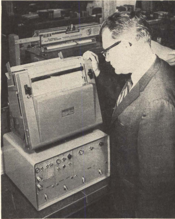
Paper facsimile recorder is Alden dual mode model 9225. Muirhead and Fairchild Camera machines also may be employed.
