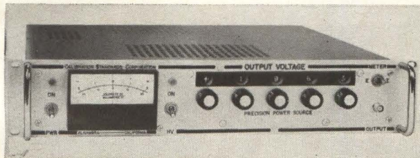
Digital power supply gives 0.005% per day and 0.02% per year stability at voltages between 0000 and 2111 volts d-c. The device may be used as a multiplier photo tube supply, an ionization-chamber supply, a klystron supply, or a backward wave oscillator supply, according to the manufacturer, the Calibration Standards Corp., Alhambra, Calif.
