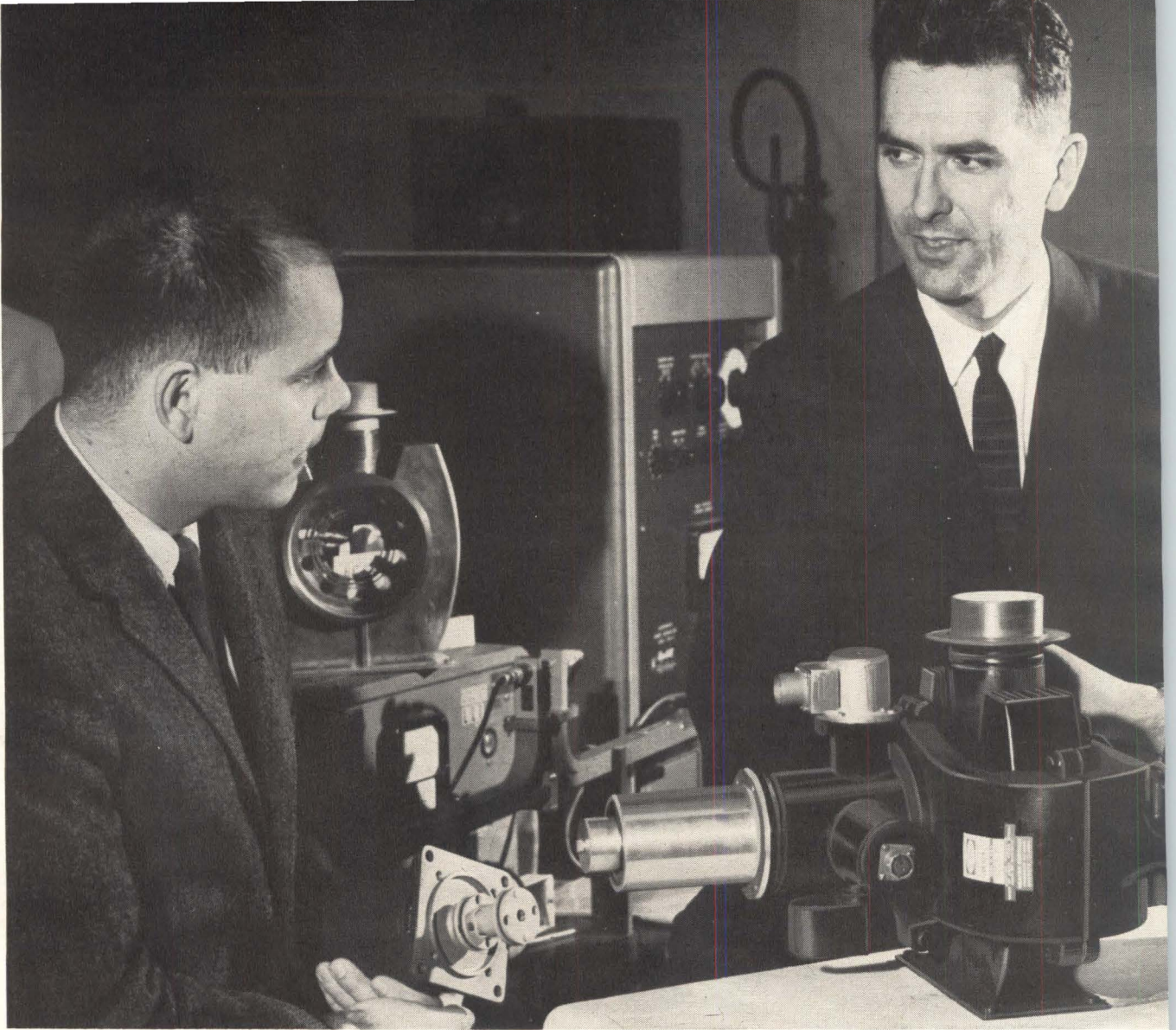
Tuned magnetron being examined by S. Ameen (right) is tuned by motor held by J. Butler (left) while the author looks on. All are section heads at Raytheon's Spencer Laboratory.
