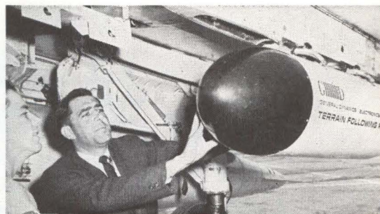
COMPACT terrain-following radar in pod attached here to Navy's A4C Skyhawk has also been tested by USAF
