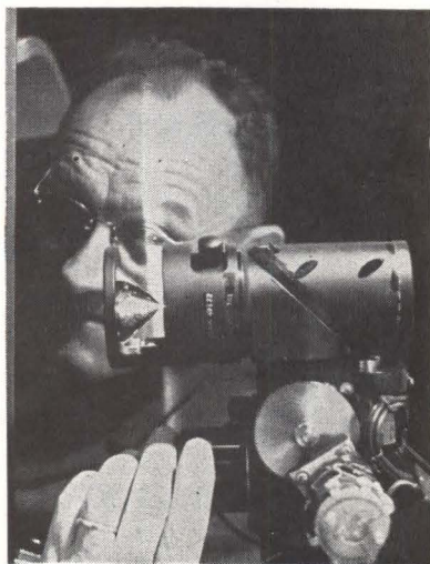
HORIZON projector generates an artificial horizon of light around pilot at all times, kept parallel to earth's horizon by vertical gyro commanding pitch and roll drive servos—Fig. 2
